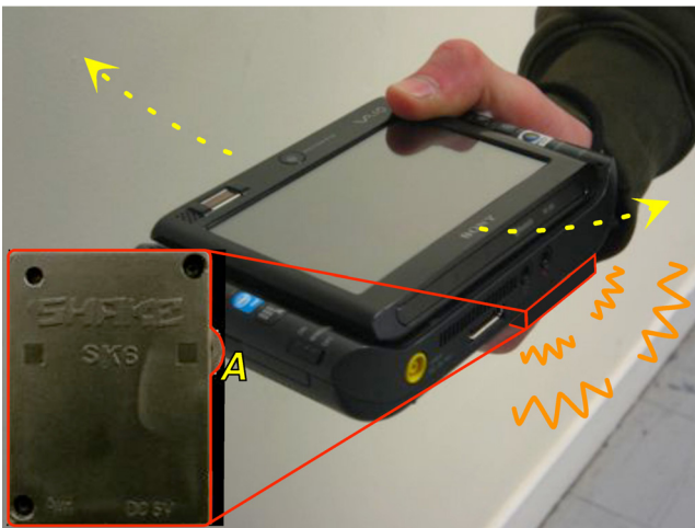
Figure 1: The haptic system in use: the SHAKE device (shown inset) vibrates when the user points toward a location with geo-tagged content available. Pressing the SHAKE's navigation button (shown at A) selects the target.
