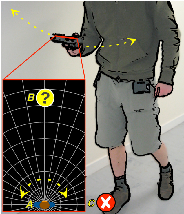
Figure 3: The visual system in use for the study, showing inset the display the user sees. The user is represented on the screen by the icon at A and a highlighted target is shown at point B. The icon used for unselected targets is shown at C.
