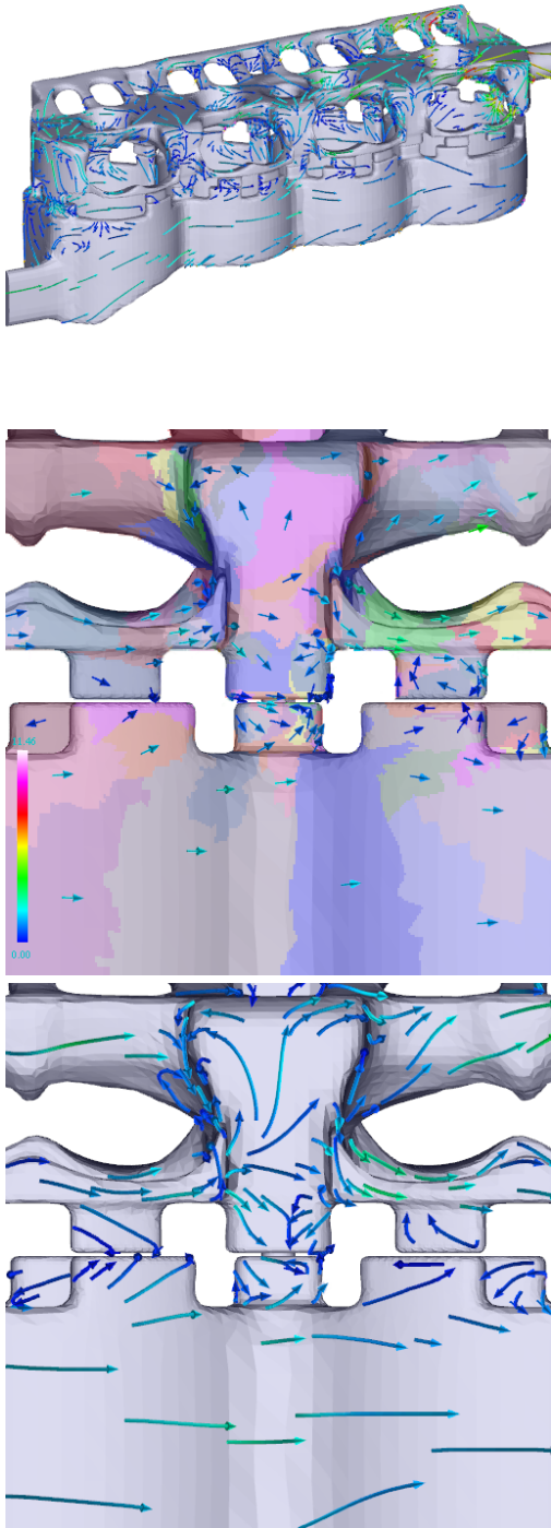
Fig. 15. Various visualization options applied to depict vector field clusters on the cooling jacket surface - a composite of 228k unstructured, adaptive-resolution polygons: (top) the glyph visualization illustrating an overview of the flow field on the surface using \epsilon = 25\% , (middle) the glyph visualization and (bottom) the cluster-based streamlet visualization providing a close-up view on the area deemed interesting with \epsilon = 38\% and \epsilon = 35\% .
