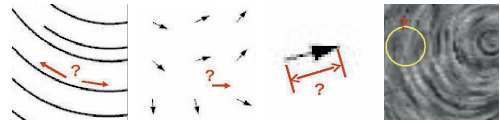
Figure 2: Sources of error in flow vis. (left to right): missing information, interpolation, quantization, noise
