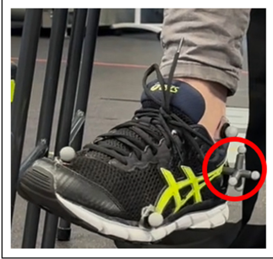
Figure 4. Detail of the three-point calcaneal marker cluster inserted through a shoe aperture, ensuring direct skin contact for accurate tracking of foot motion relative to the shoe.
