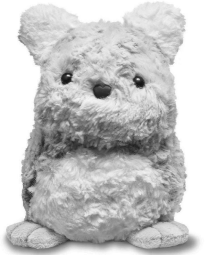
Fig. 1 | Purrble: socially assistive robot intervention device. Image of the socially assistive robot provided to participants in the intervention condition. Interactive features include touch-responsive sensors in the ears, feet and back stripe, a gyroscope for movement detection and an internal vibration motor that generates heartbeat-like and purr-like sensations.
