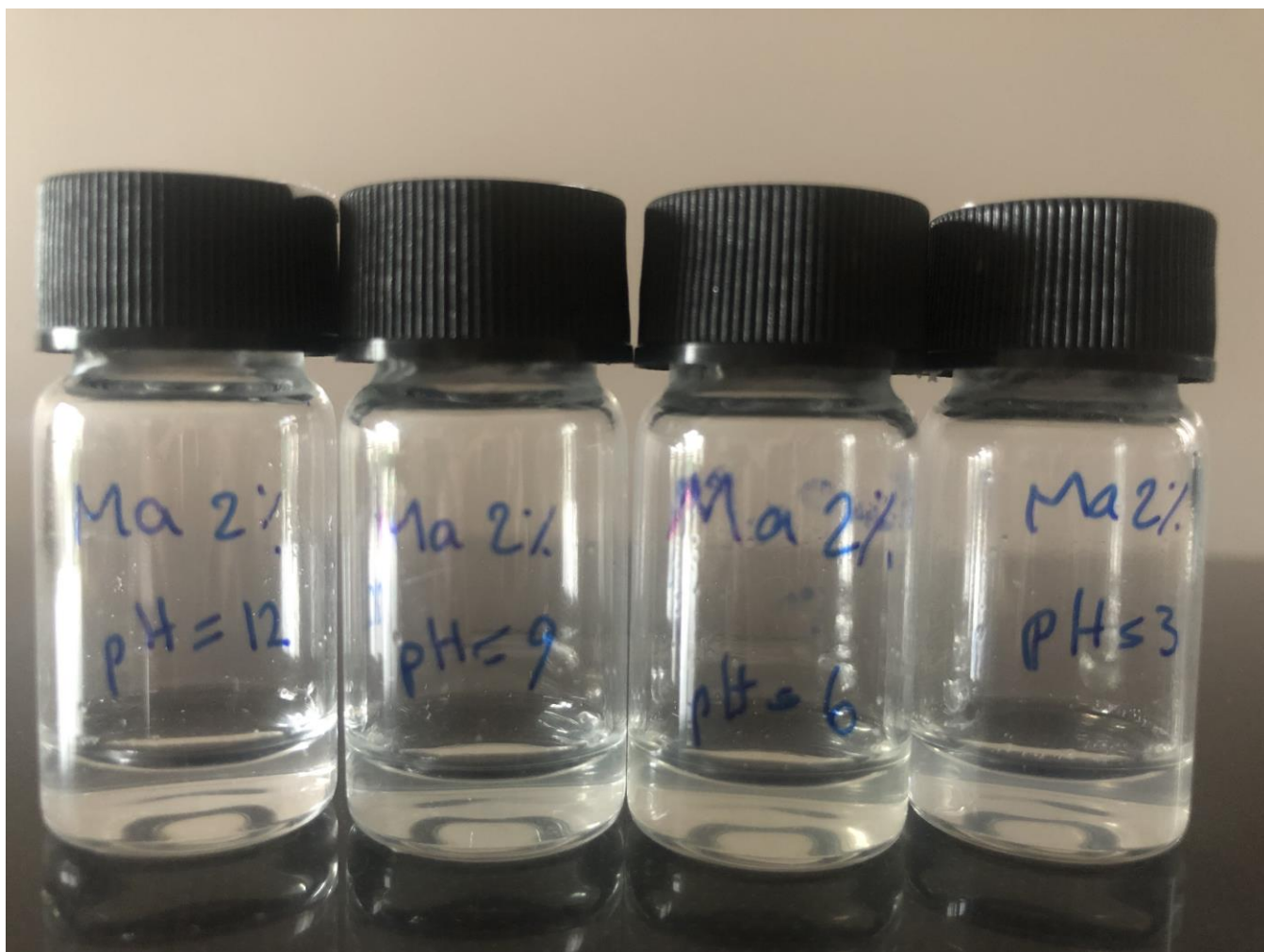
Fig. E.4: shows a separate pH screening series for MA- \text{alt-C}_{18} -g-PEG at 2% w/w, with pH values ranging from 3 to 12. These samples were used to assess micelle stability and visual clarity across acidic, neutral, and basic conditions.
