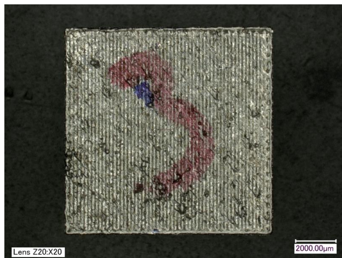
Figure 4:23: Top of Exposure Time 130 \mu\text{s} , Laser Power 200W, Meander Laser Pattern, x20 mag
