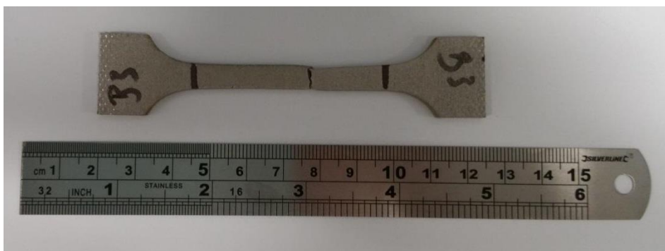
Figure 4:50: Extension of 90° rotation and meander laser patten, 130µs exposure time and 180W laser power sample, UTS 578 MPa
