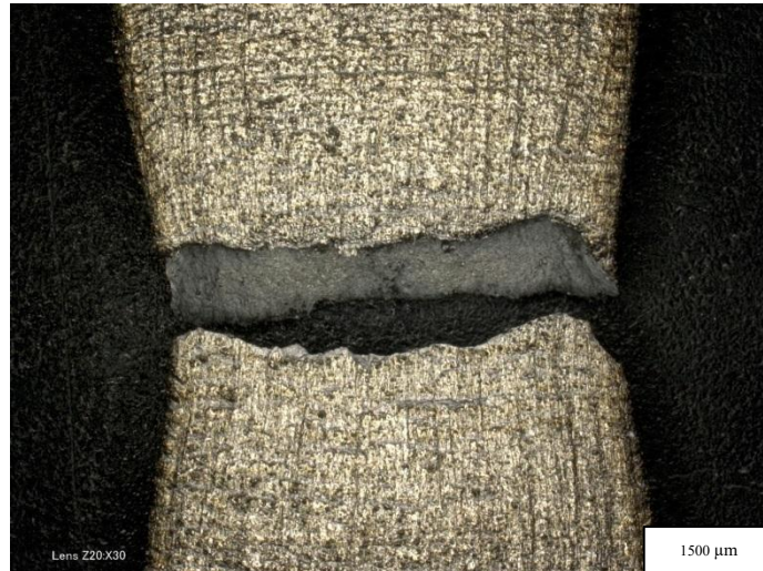
Figure 4:61: Build 17 Vertical, Meander Laser Path, Exposure Time 80 \mu s, Laser Power 200W, Heat Treatment 1 Applied, UTS 645 MPa
