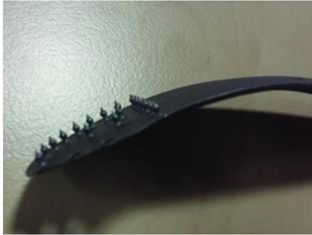
Figure 2:5: Metal pins to attach AM parts to composites [57]
