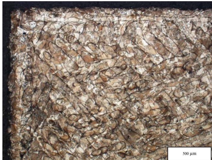
Figure 4:108: Laser Pattern of 67° Rotation Meander Cube
