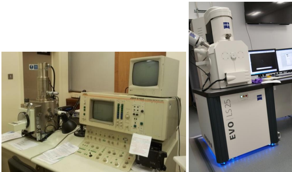
Figure 3:16: Scanning Electron Microscopes Used (a) Jeol6100 SEM, (b) Zeiss EVO LS25 SEM
