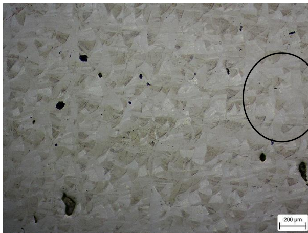
Figure 4:112: 67° Rotation, Meander Laser Path, Exposure Time 130μs, Laser Power 200W
