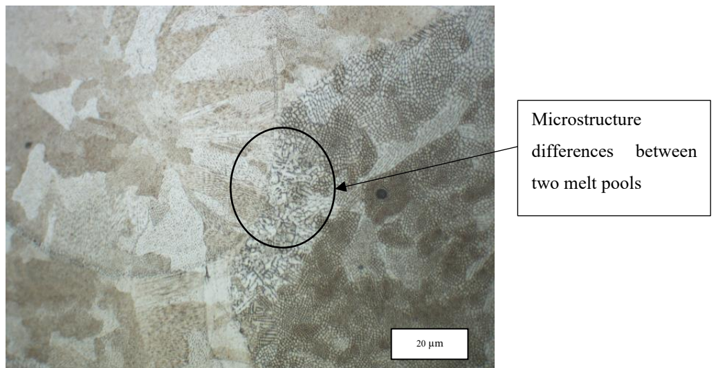
Figure 4:109: Microstructure of an AM SS316L Cube
