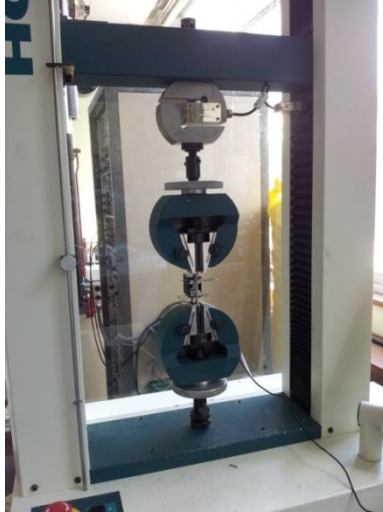
Figure 3:13: Tensile test set up of both the Hounsfield and Tinius Olsen Tensile Test Machines
