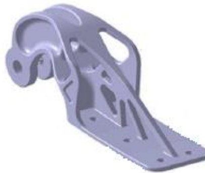
Figure 2:7: Optimised A320 Nacelle Hinge Bracket [16]
