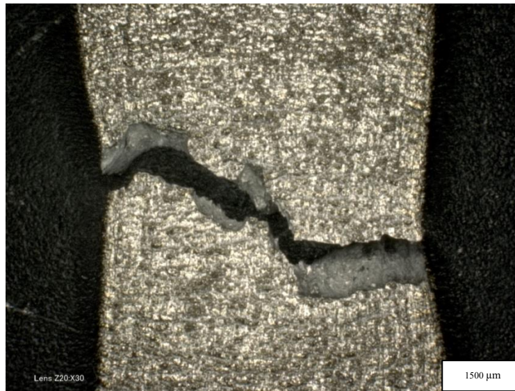
Figure 4:60: Build 17 Vertical, Meander Laser Path, Exposure Time 80 \mu s, Laser Power 200W, As Built, UTS 615 MPa
