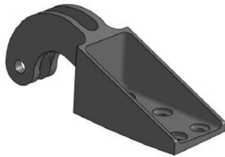
Figure 2:6: Original A320 Nacelle Hinge Bracket [16]
