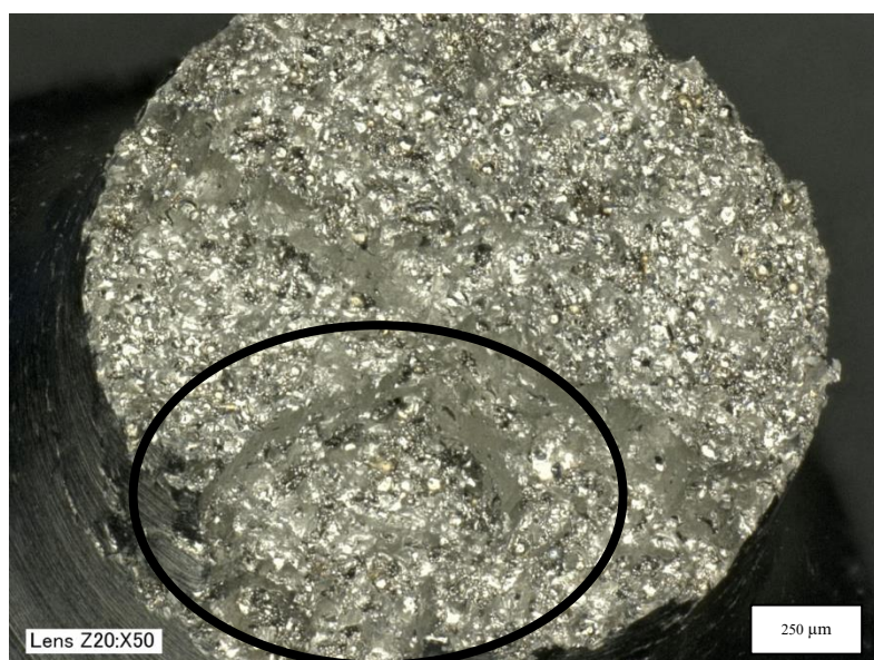
Figure 4:79: Build 25 Vertical, Meander Laser Path, Exposure Time 80μs, Laser Power 200W, Machined from Round Bars
