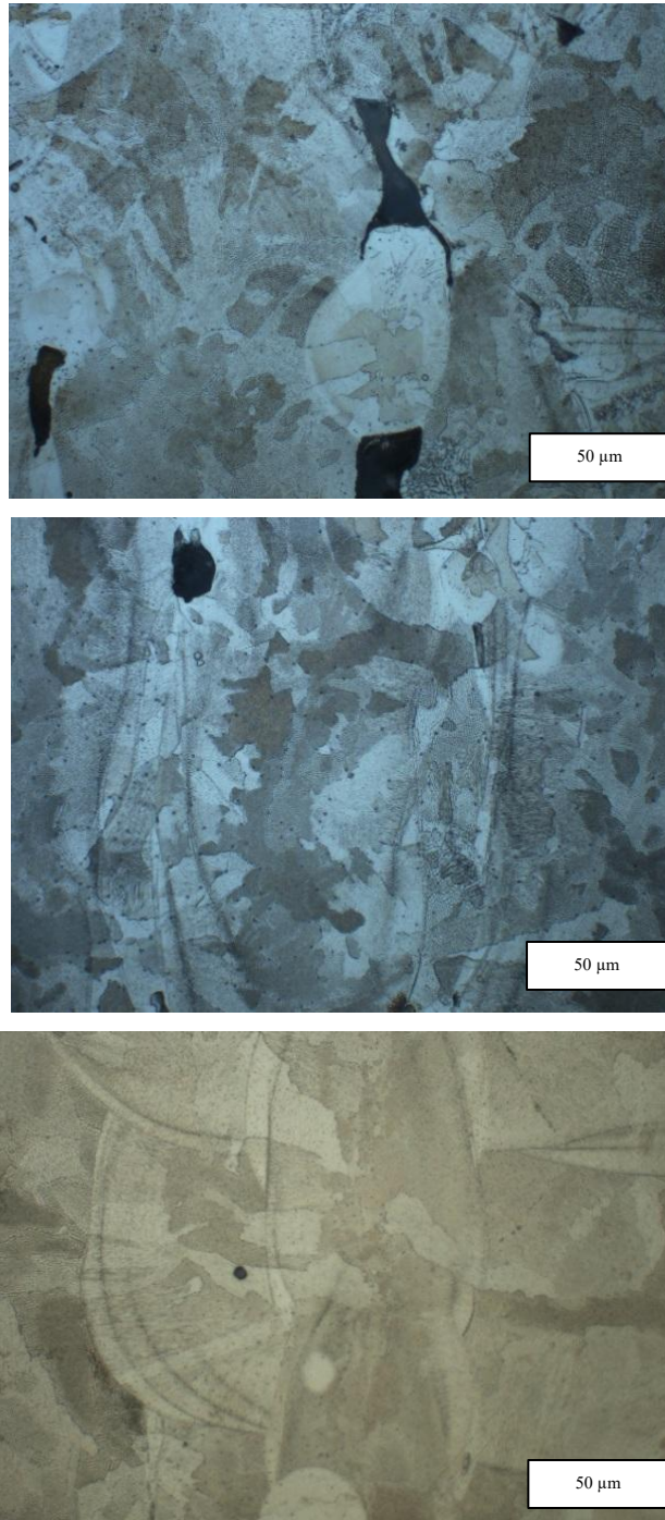
Figure 4:102: Microstructures of the 90° Stripe Cubes, within a layer (a) 80μs exposure time and 160W laser power, (b) 105μs exposure time and 180W laser power, (c) 130μs exposure time and 200W laser power
