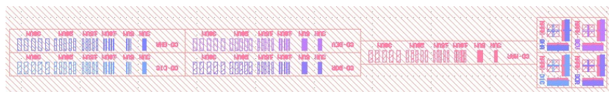
Figure 69. New alignment marks format, presented here horizontally, however are in the vertical orientation on the mask
