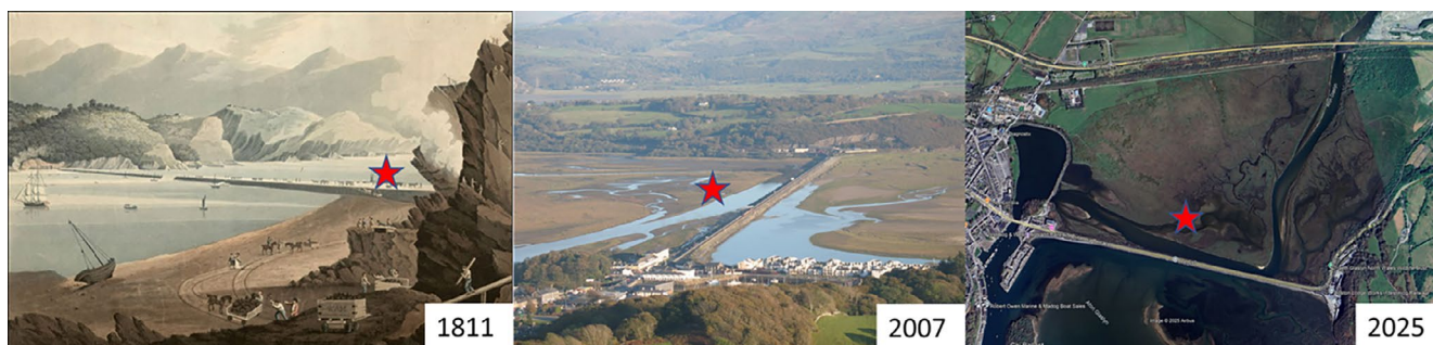
FIGURE 5 | Reclamation of the Glaslyn estuary involved the construction of a 1.4 km embankment known as the Cob. That led to the creation of extensive farmland and the development of Porthmadoc as a town and port. Image credit: 1811 National Library of Wales, 2007 Peter Humphries and 2025 Google Earth.
