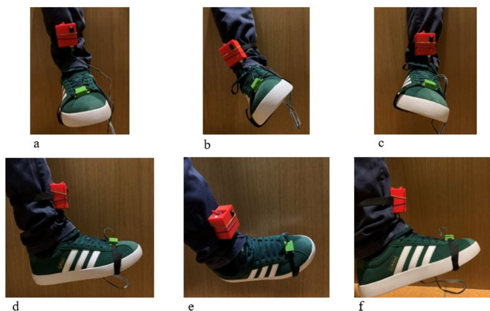
Figure 8. Ankle eversion and inversion. Frontal view: (a) neutral, (b) maximum inversion, (c) maximum eversion; lateral view: (d) neutral, (e) maximum inversion, (f) maximum eversion.
