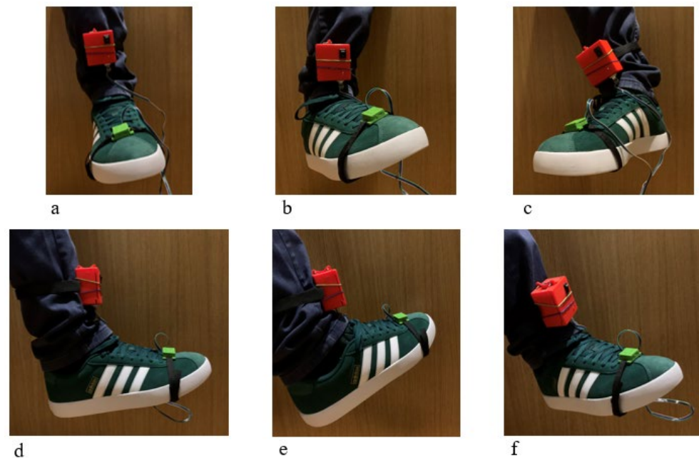
Figure 9. Ankle abduction and adduction. Frontal view: (a) neutral, (b) maximum adduction, (c) maximum abduction; lateral view: (d) neutral, (e) maximum adduction, (f) maximum abduction.
