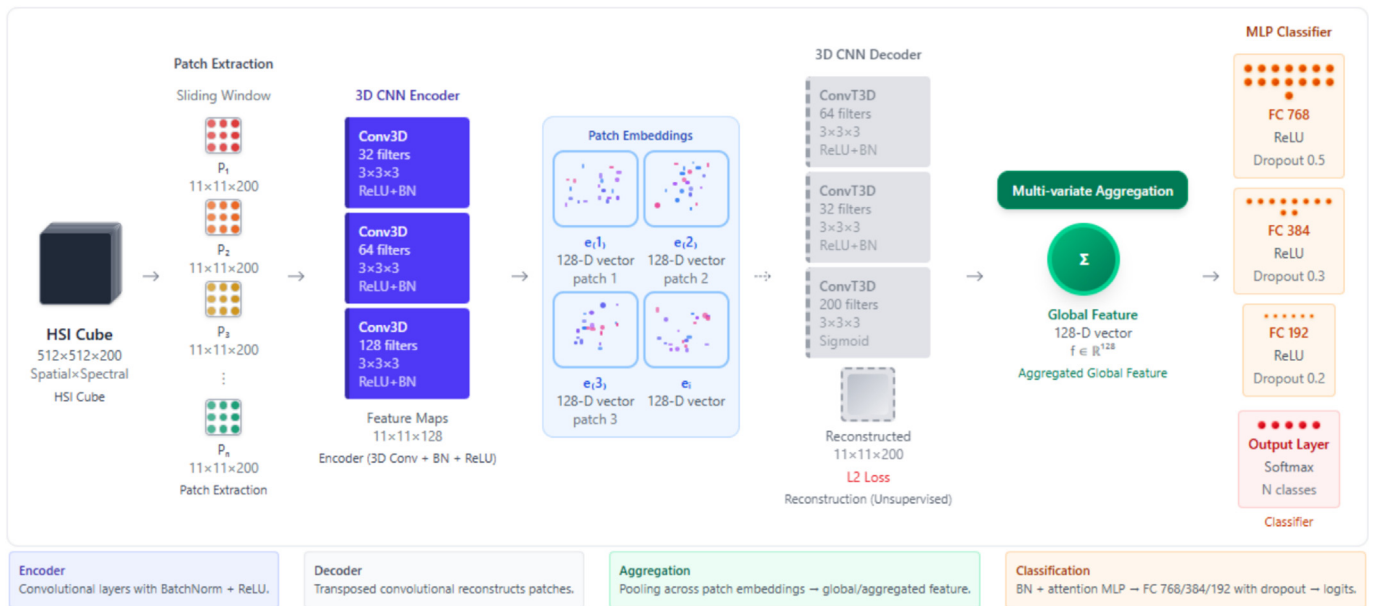
Fig. 2. Overview of the proposed 3D-CNN-based framework for hyperspectral image (HSI) classification. Spatial-spectral patches are extracted from the input HSI cube ( 512 \times 512 \times 200 ) using a sliding window approach. These patches ( P_1, P_2, \dots, P_n ) are passed through a 3D-CNN encoder composed of convolutional layers with batch normalization and ReLU activations to generate compact patch embeddings (128-D feature vectors). The encoder is trained in an unsupervised manner via reconstruction, where a 3D-CNN decoder attempts to reconstruct the original patch with an L_2 loss. After training, the patch embeddings are aggregated through a multi-variate pooling mechanism to obtain a global feature representation (128-D). Finally, the global feature is passed through a multilayer perceptron (MLP) classifier with fully connected layers, ReLU activations, and dropout regularization, followed by a softmax output layer to produce class predictions.
