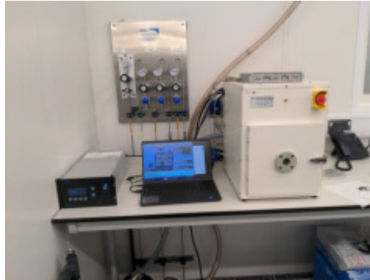
Figure 3.3: PE-50 Plasma asher sold by Plasma Etch. This tool was used to de-scum the sample after the photoresist was developed. This is to remove contaminants in the developed regions. This uses an O_2 plasma to do this. This is a light etching process to remove contaminants from the surface rather than etching into the sample.
