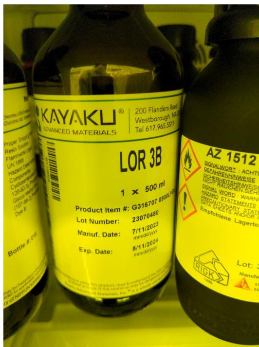
Figure 3.24: LOR 3B positive photoresist, produced by Kayakli, for bi-layer photoresist processes. This was used as part of a bi-layer, metal lift-off process.
