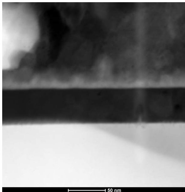
Figure B.15: Here is one of the TEM images used in this work, this is a cross-section of \beta -Ga 2 O 3 /Al 2 O 3 sample. This was used to determine the thickness of the Al 2 O 3 layer. This was using the scale and ImageJ and the tabulated data is seen in table B.7. In this table it is TEM image 7
