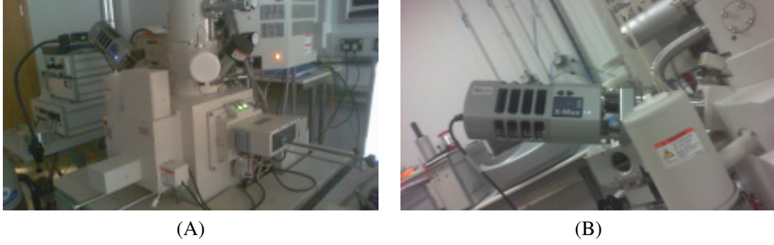
Figure 3.19: The SEM used in this work, (A) is the Hitachi S-4800 SEM and (B) is the Oxford instruments EDX detector.
