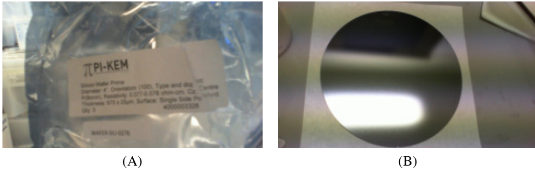
Figure 3.33: Si wafers used in this work, (A) is an example of a 4" wafer this was at test grade and (B) a 12" wafer which is dummy grade. Test grade wafers were used in dry runs, optimisation, and prime grade wafers for spectator wafers, and dummy grade wafers were used as carriers, or initial process testing.
