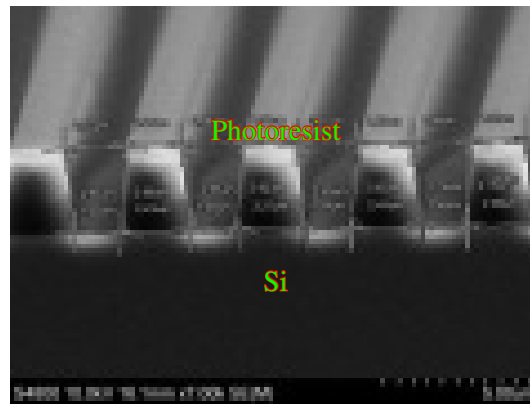
(C) Vacuum contact Noticeably better than soft contact.
