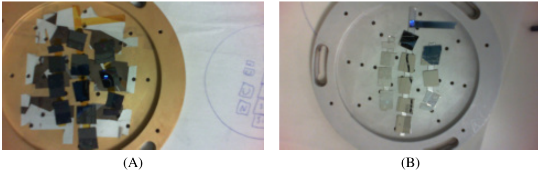
Figure 3.10: An example of small samples being held in the PVD, before (A) and after (B) the deposition. This has to be done using polyimide tape or clips.
