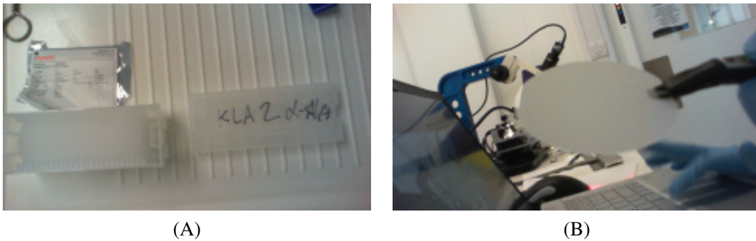
Figure 3.32: One of the sapphire \alpha -Al 2 O 3 wafers used in this work, these were purchased from Inseto. These were 2", double side polished prime grade wafers orientated on the c-plane (0001), these were grown with the Kyropoulos method. Kyropoulos is similar to the Czochralski however the gradient of the heating is more gradual.
