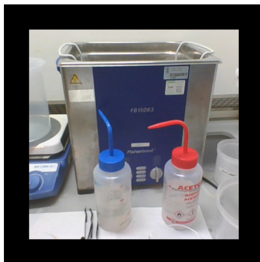
Figure 3.2: The sonicator used in this work, this was used for solvent cleaning as well as some lift-off procedures. This is a bath which applies a high frequency agitation, which can be used to physically dislodge and dissolve particles into a solvent. This is not always used as it can cause some level of damage to samples.
