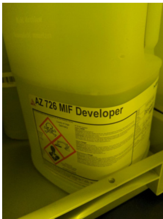
Figure 3.28: AZ 726 developer, a TMHA based developer used in this work.
