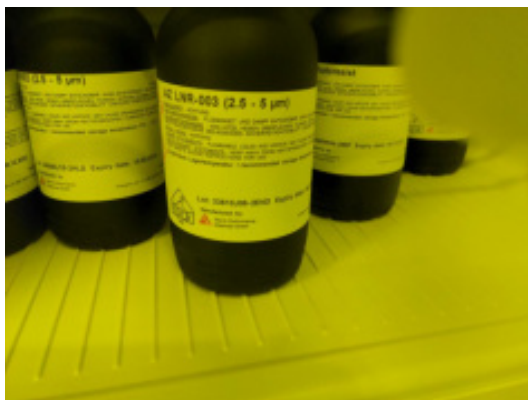
Figure 3.23: AZ LNR-003 negative photoresist, this was used for lift off processes in this work.
