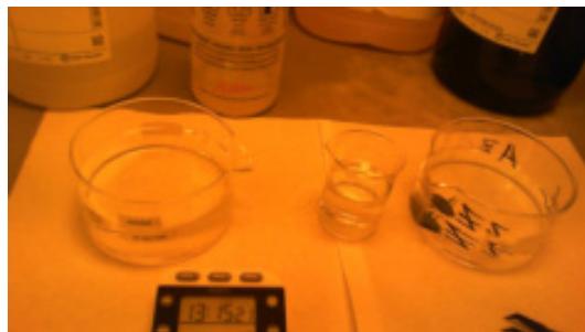
Figure 6.8: The development set-up used in the developer optimization, this was one of the experiments made as part of the developer trial. It was found that the development in larger beakers outperformed those in smaller beakers.
