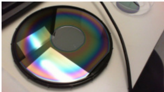
Figure 3.14: This is the carrier wafer which had to be fabricated in order to process the 2" \text{Ga}_2\text{O}_3 samples. This was done using both the PECVD to create a carrier wafer to securely hold samples.
