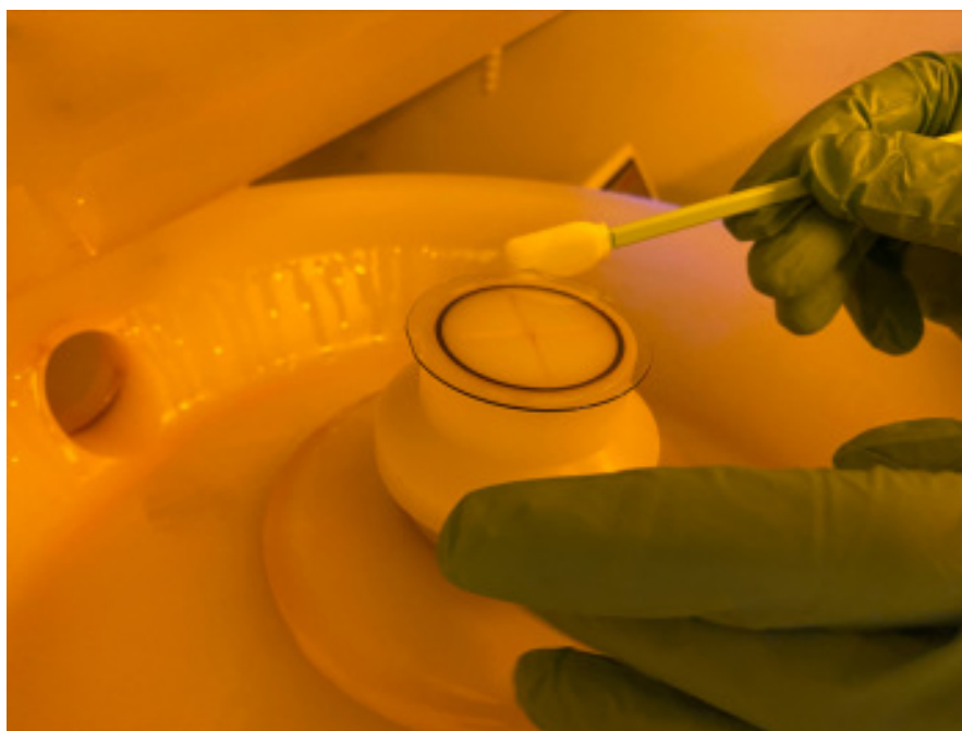
Figure 5.3: Manual removal of the edge bead. This was done with a swab dabbed in acetone and then lightly brushed around the edge of the sample.
