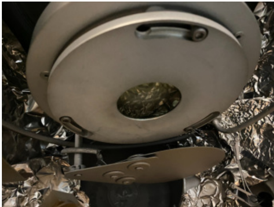
Figure 3.9: The 2" holder which had to be made for this tool in order to hold 2" wafers without the need for tape. This is a simple holder with a small inlay to hold a wafer without the need for clips or polyimide tape. This results in a
