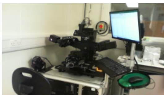
Figure 3.20: The Ellipsometer used in this work, the M-2000 Spectroscopic Ellipsometer by J. A. Woollam Co. Predominately this was used to determine and confirm the thickness of photoresist which was spun onto the surface of predominately Si. This was often the first stage of optimising the protocol for a particular photoresist.
