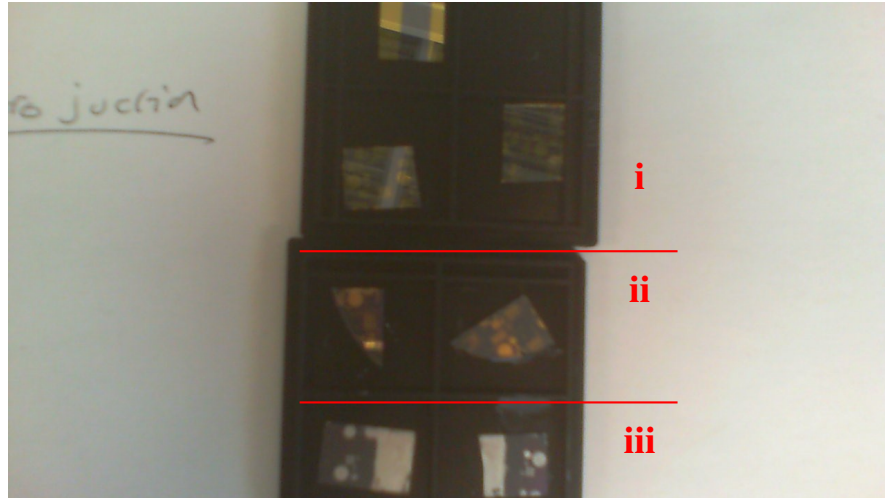
Figure 6.3: The \beta -Ga 2 O 3 /Si heterostructure samples after the metal deposition metal lifted off. The metalisations were Ti/Au (i), Ti/Ag (ii) and Ti/Al (iii).
