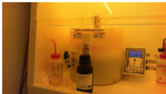
Figure 3.5: One of the Laurell spin coaters used in this work, this was used in all processes which require a photoresist spun on to a sample, or adhesive agent. Depending on the process the parameters can be changed from spin speed, acceleration, duration, a process can be multiply steps. It is able to hold wafers up to 200 mm with adaptors down to 10 mm.
