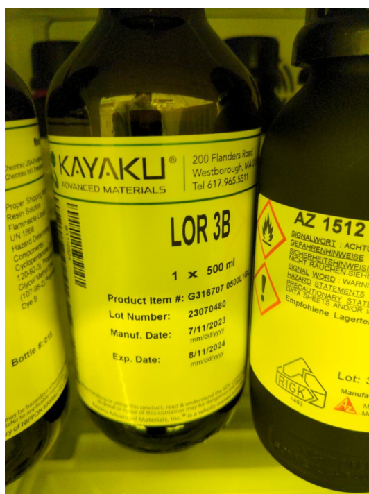
Figure 3.25: AZ 1512 HB, a positive photoresist, produced by MicroChemicals, used in a bi-layer photoresist processes. This was used as part of a bi-layer, metal lift-off process.
