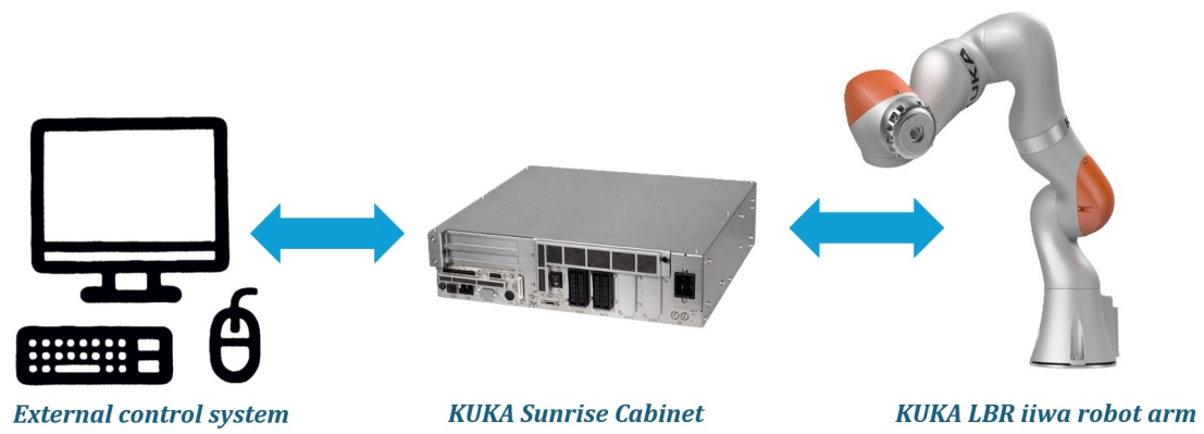
Figure 2.7: Control and communication of the robot via the KUKA Sunrise Cabinet.
