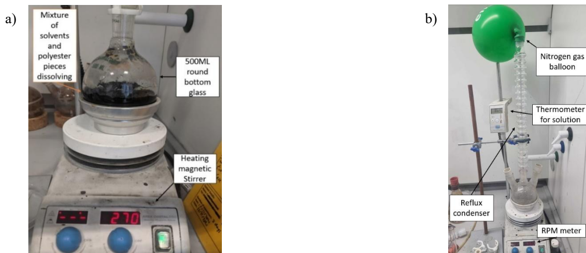
Figure 23 a) Dissolution of polyester plastic utensils. b) Reflux system for dissolution
