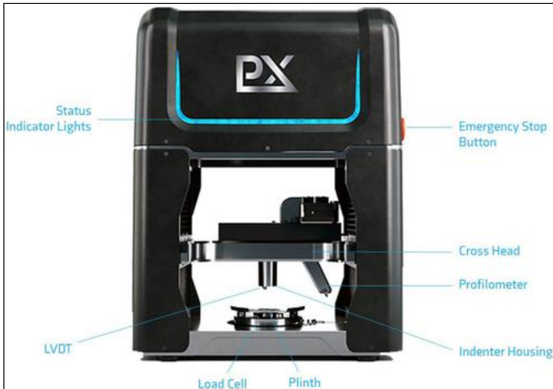
Figure 58- Labelled diagram of plastometer[131].
