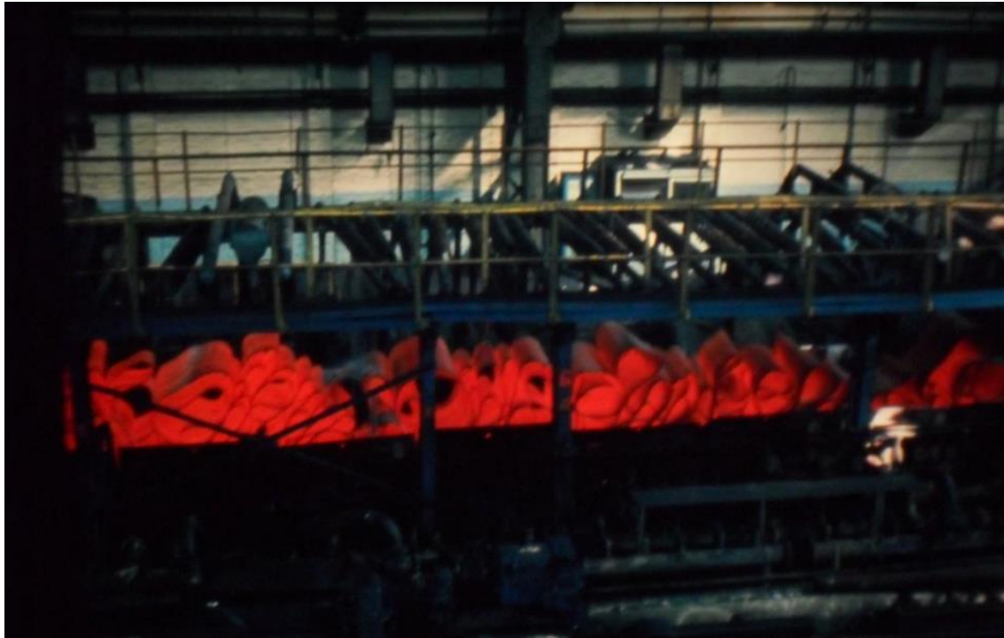
Figure 24- Example of hot mill 'Cobble'[81].
