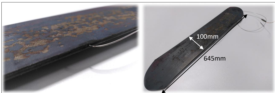
Figure 84- Previously hot rolled DP800 strip, with k-type thermocouple mounted in the centre.
