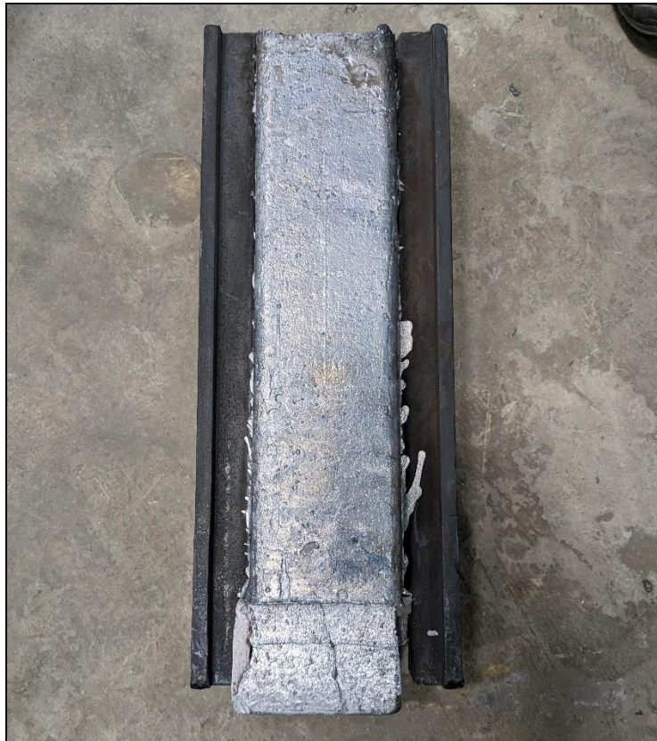
Figure 44- VIM cast material in one half of refractory cast.
