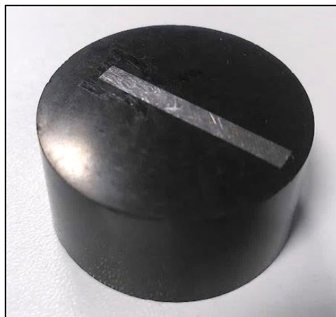
Figure 52- 30mm sample mounted in conductive resin for microscopy.
