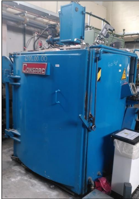
Figure 38- A photo of the Consarc VIM used to manufacture DP800 blocks for hot rolling.
