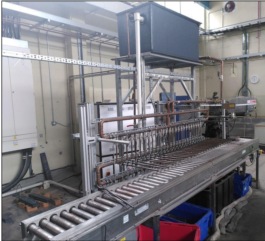
Figure 42- Photo of SAMI ROT with water top water headers visible and wate tank above.
