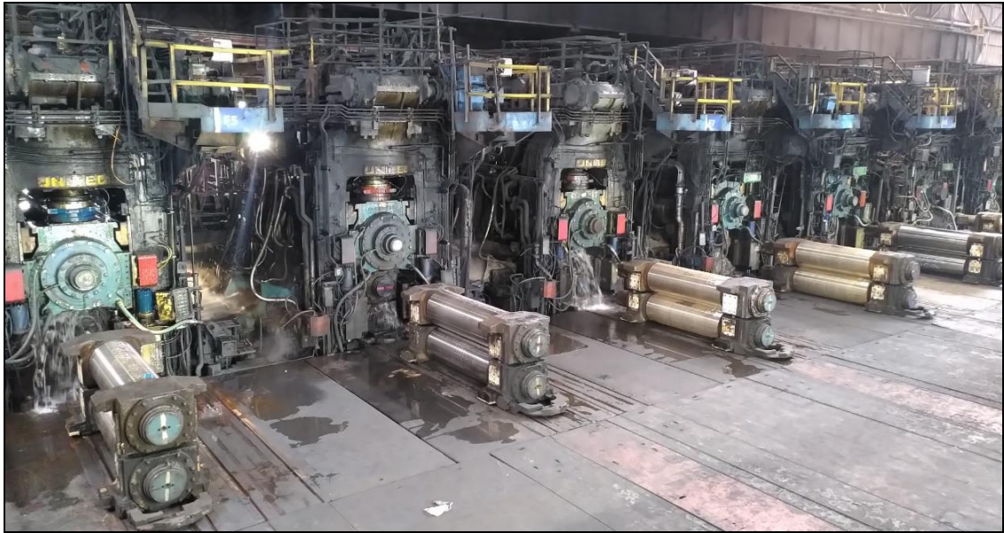
Figure 22- Tata Steel Port Talbot finishing mill stands, with replacement rolls ready for changing to minimise mill down time.
