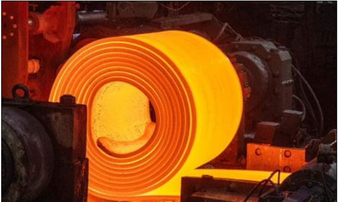
Figure 21- A coil of 'transfer bar' on the coil box awaiting entry into the finishing mill[80].
