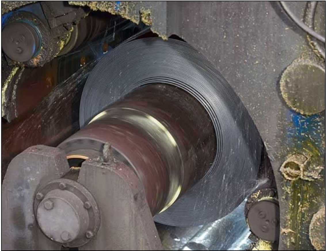
Figure 29- Photo of a Downcoiler accumulating hot rolled strip[89].
