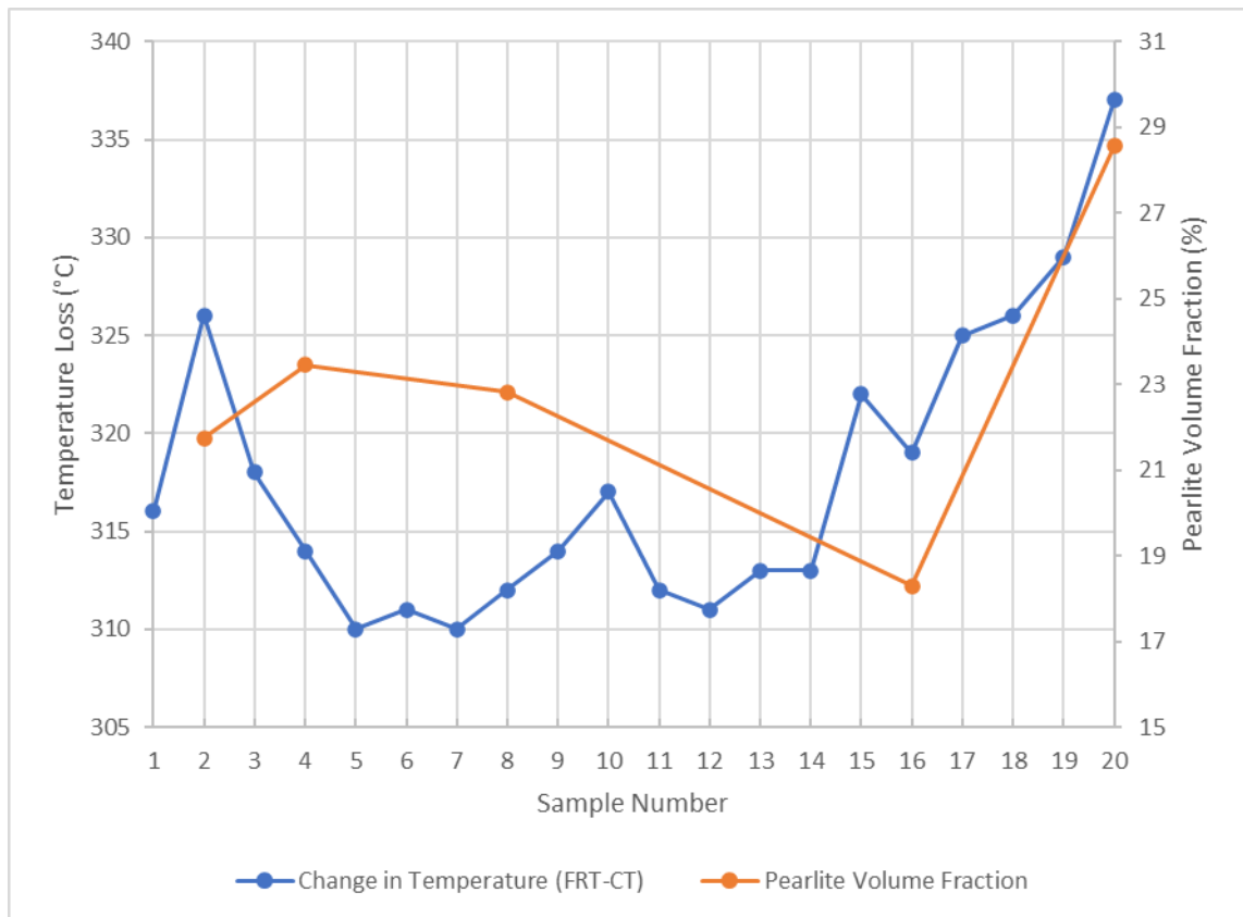
Figure 71- Comparison of temperature change over ROT (FRT - CT) and measured pearlite volume fraction for samples 2, 4, 8, 16 and 20.
