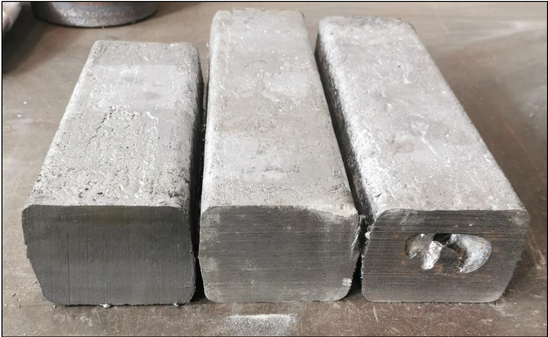
Figure 45- VIM cast ingots cut for manufacture of blocks for hot rolling.
