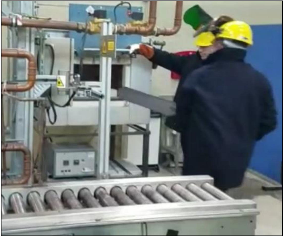
Figure 60- Operators placing rolled sample into 'coiling' furnace for a slow cool.
