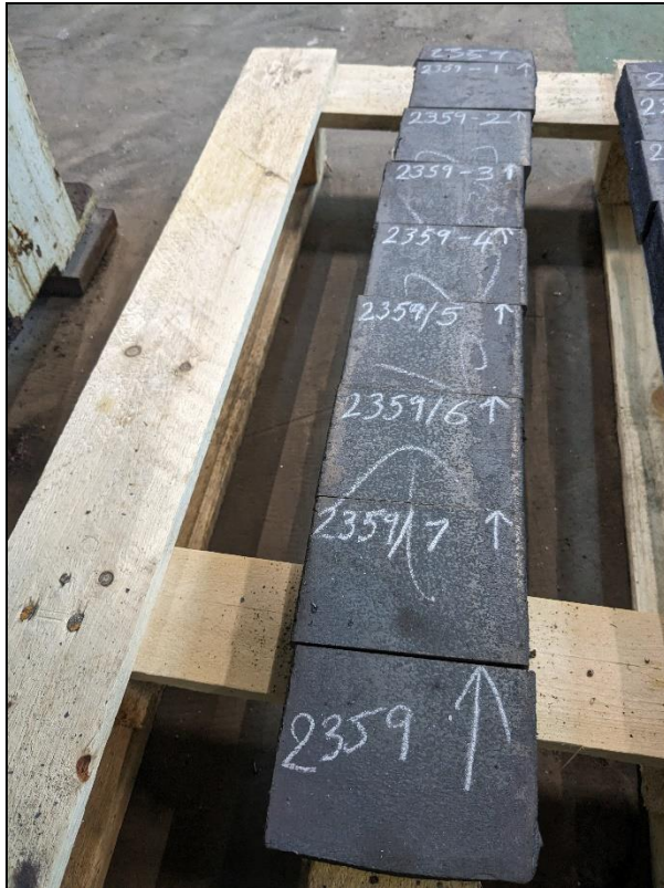
Figure 46- 'Transfer bar' cut ready for hot rolling, with coil ID rolling direction marked.
