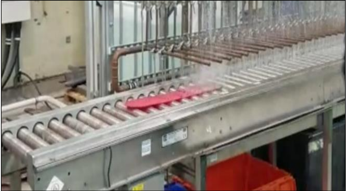
Figure 59- Hot rolled sample entering the ROT water sprays.
