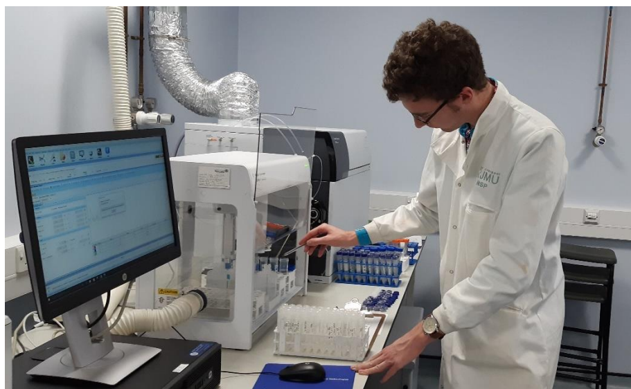
Figure 2-3 – an Agilent Technologies ICP-MS 7900 in use for this project at Liverpool John Moores University. The ICP-MS itself is to the rear with the silver corrugated extractor hose attached, then being pointed at by the author is the autosampler and prepared samples, and then the computer and Agilent Technologies software to control the system.
