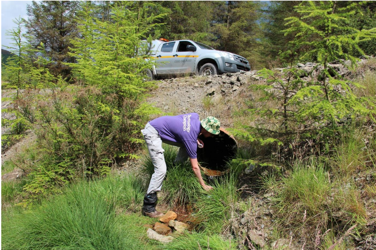
Figure 2-1 - An ideal site for the bucket and stopwatch method of flow measurement at Nantymwyn, as the flow is concentrated into a culvert with a large enough fall to accommodate a bucket. Sampling site reference number 88224
