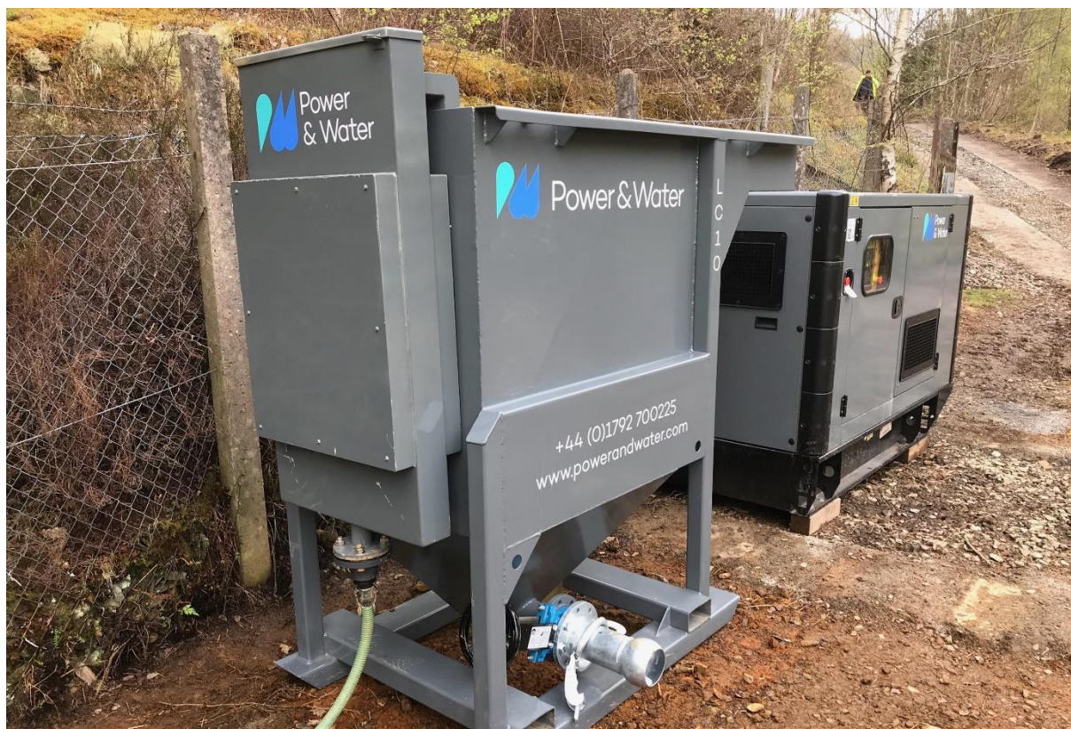
Figure 2-7 - the portable Power & Water electrolysis plant at Cwm Rheidol, with generator behind. Picture courtesy of Power & Water
