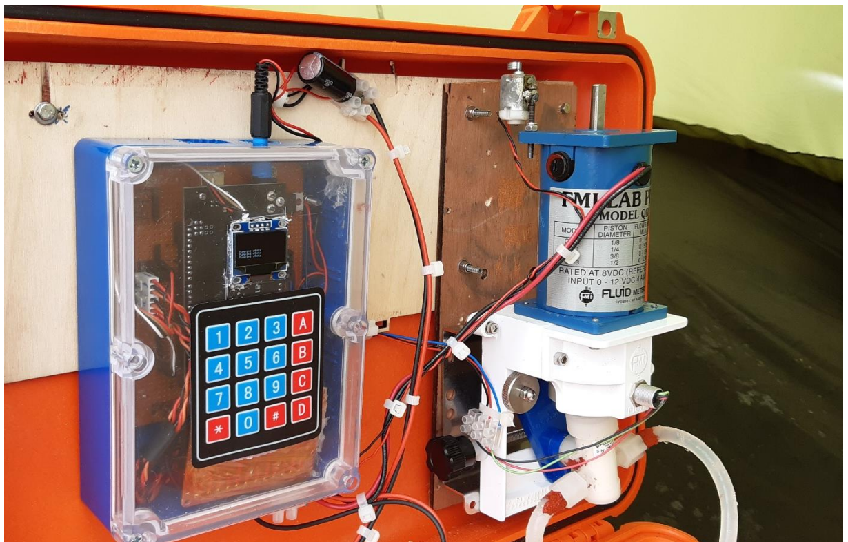
Figure 4-7 - computer controlled peristaltic pump, with controller, pump, (battery out of sight), and flexible piping to the tracer tank, and to the Nant y Bai
