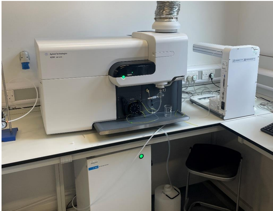
Figure 2-4 - an Agilent Technologies MP-AES 4200 at Swansea University
