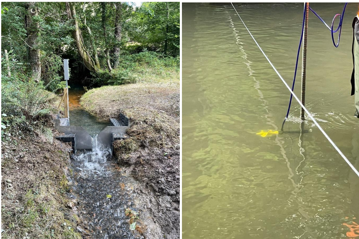
Figure 2-2 - left, V-notch weir with a constant depth logger at Nantymwyn (sampling site reference number 88204); right, an impeller type flowmeter, with graduated depth marked on the vertical support for the flow meter, and distance across the channel measured from the horizontal tape measure
