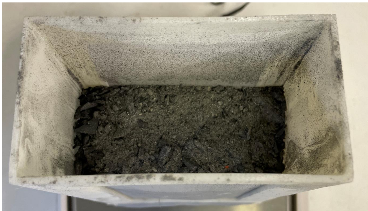
Figure 2-9 - biochar in a porous container, allowing water to pass through the biochar for treatment, but retaining the biochar (and metals it removes) within the container. The container opening is approximately 2cm x 6cm, and 10cm tall.
