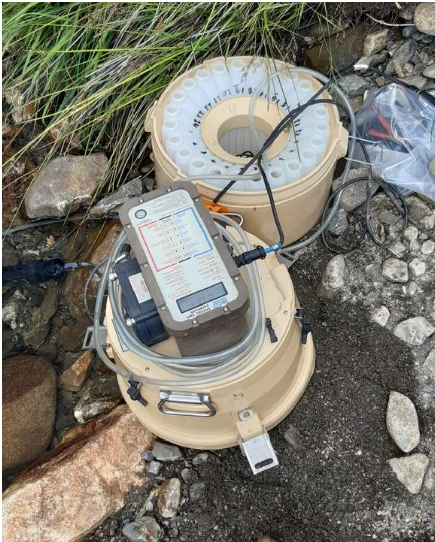
Figure 2-5 - An ISCO 3700 automatic watersampler in use on the Nant y Bai
