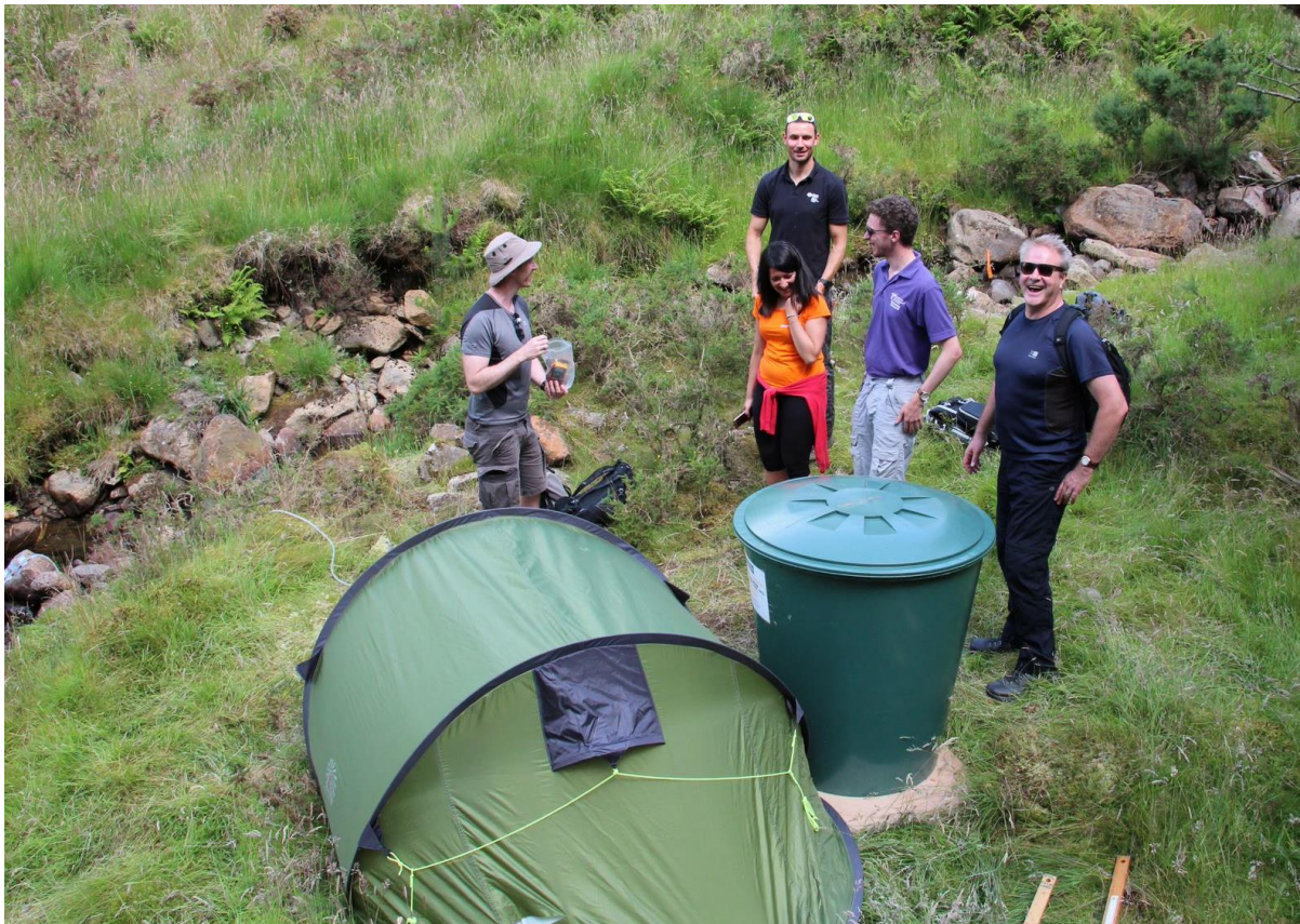
Figure 4-4 - Tracer injection tank, with pump and pump controller shielded in the tent. The injection pipe can be seen running towards the Nant y Bai stream
