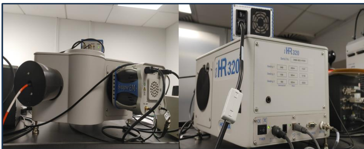
Figure 5.13: Photo of Horiba iHR320 Raman spectrometer.
