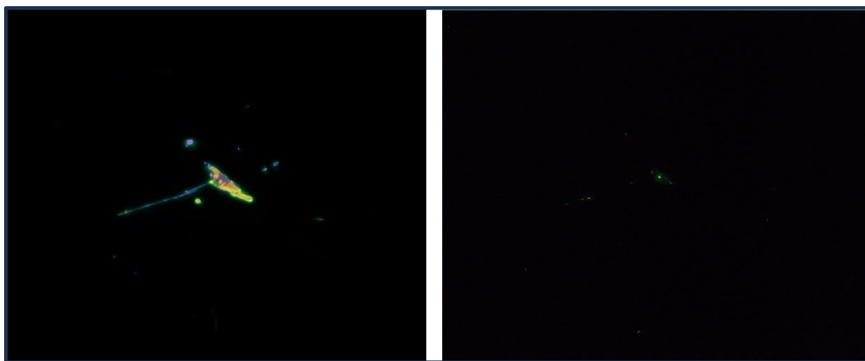
Figure 7.23: PL intensity before water treatment Figure 7.24: PL intensity after water treatment (Scale: 50 \mu\text{m} )
