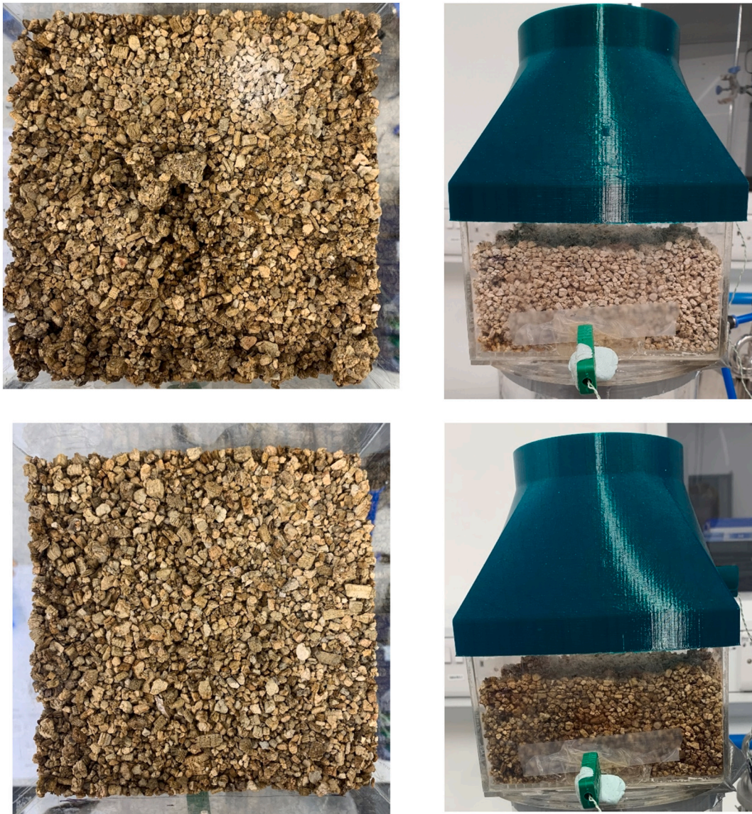
Fig. 7. Images of material which is over saturated at the bottom of a 60 mm height of reactor while remaining dry at the upper surface.
