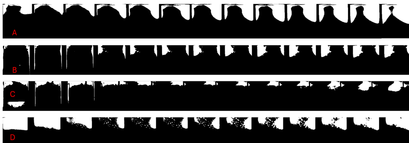
Figure 14. Thermal images taken every 10 s for the first 2 min of heating at 550^\circ\text{C} thresholded using ImageJ at a greyscale value corresponding to 60^\circ\text{C} , where (A) = the magnetite concentrates, (B) = the hematite ore, (C) = the hematite-goethite ore and (D) = sinter fines.
