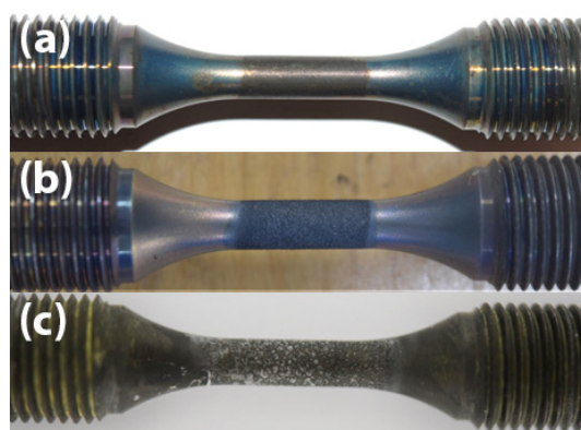
Figure 2. Surface observation after 50 h of fatigue testing in air with 0.13 mg/cm 2 of salt (a), 0.13 mg/cm 2 of salt in SO 2 (b), and 13 mg/cm 2 of salt in air (c).
