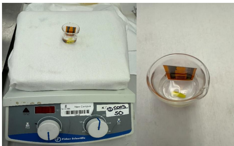
Figure 11: Overall (Left) and enlarged (Right) template removal technique with beaker, sensor, removal solution and stirrer.
