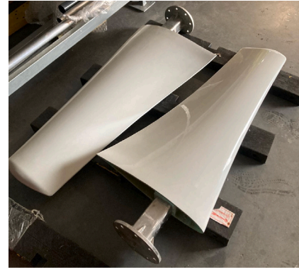
Fig. 1. (a) Design overview with components labelled (b) image of two blades, as manufactured.
