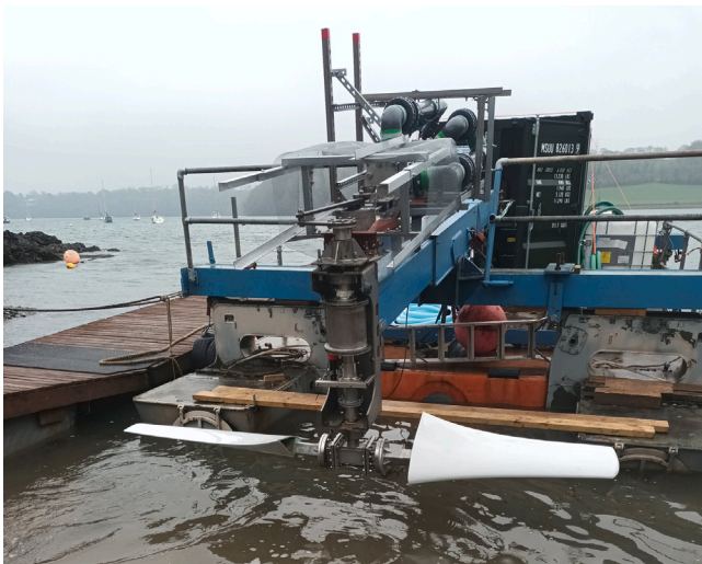
Fig. 8. Full scale turbine and pump assembled to test platform, rear view. Green control cabin to rear with the water storage IBC to the right of the cabin.
