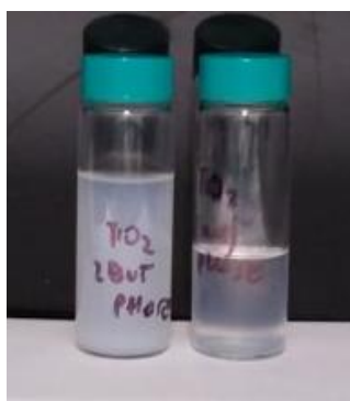
Figure 6.18: 2-butanol phase (left) and aqueous phase (right) separated after \text{TiO}_2 transfer in 2-butanol
