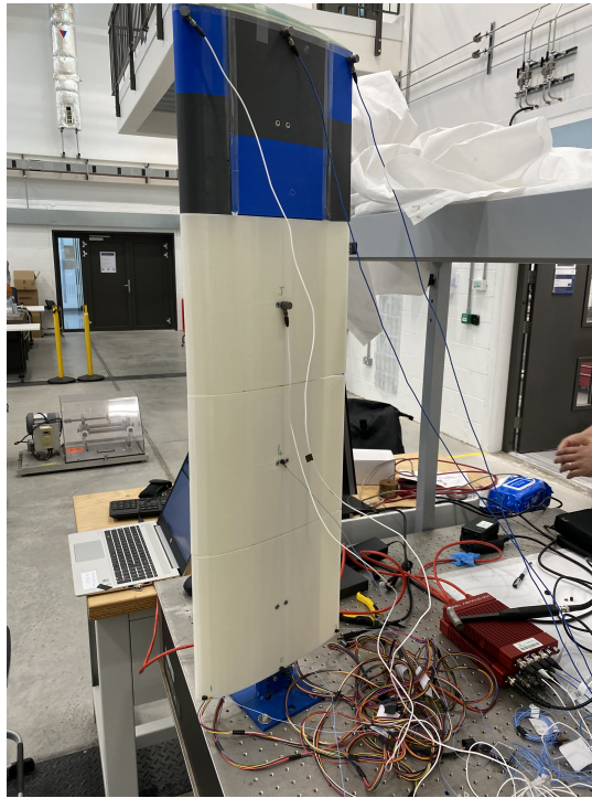
FIGURE 2.13: MODFLEX Hammer Test Setup
