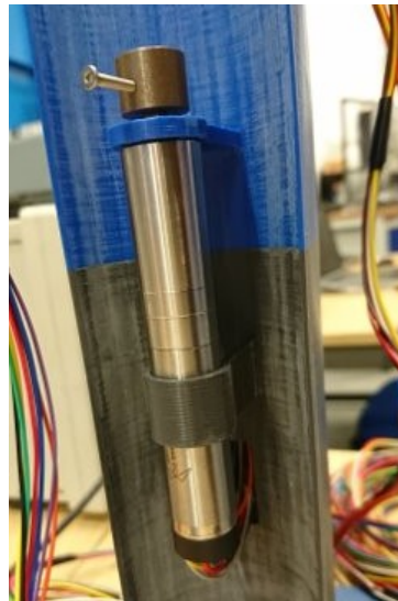
FIGURE 2.11: Maxon ECXSP16L Motor in MODFLEX wing
