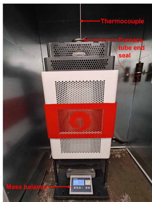
Figure 2. Carbolite Gero Ltd. high-temperature TGA tube furnace used to perform furnace replication experiments and obtain continuous thermogravimetric data.
