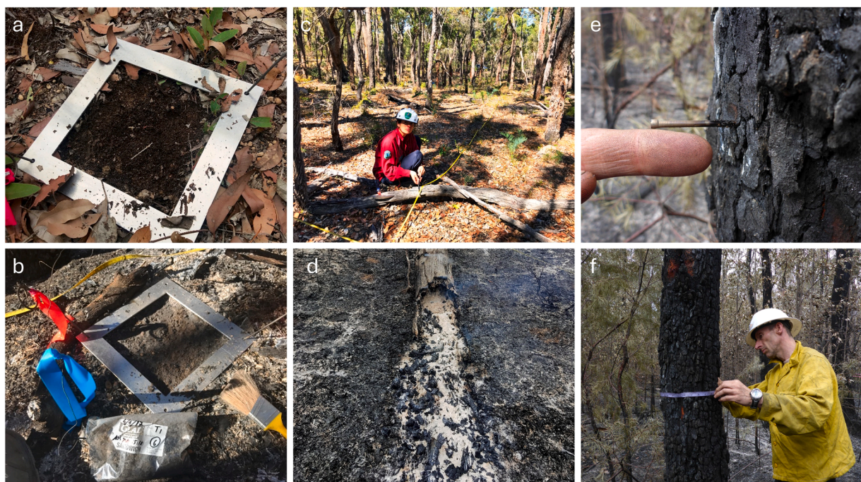
Fig. 2. Field sampling and measurements: a. sampling of pre-fire litter; b. sampling of ashes; c. quantification of down wood with the line intercept method before the fire; d. production of charcoal from a large down wood piece at Yackelup; e. nail used to re-locate tree circumference measurement; f. measurement of post-fire tree circumference.
