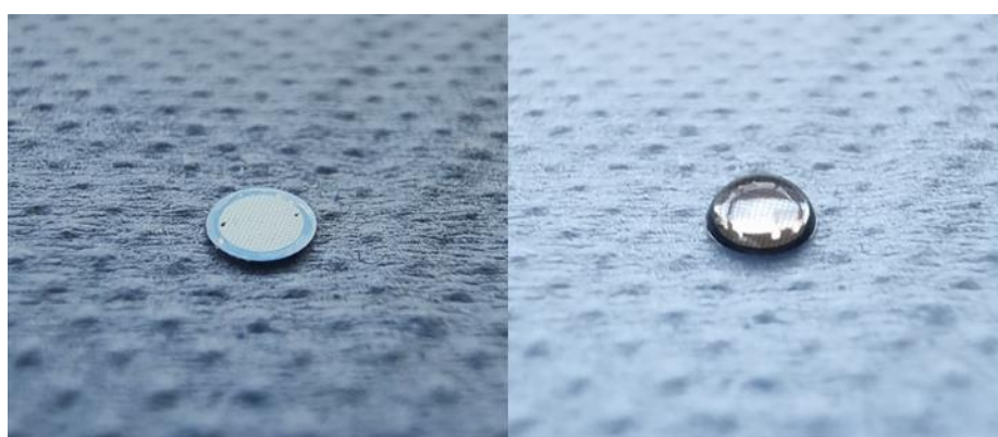
Figure 4.7 Blank TEM grid (left) and TEM grid immediately after dropcasting 5 \mu\text{L} of particle suspension (right).
