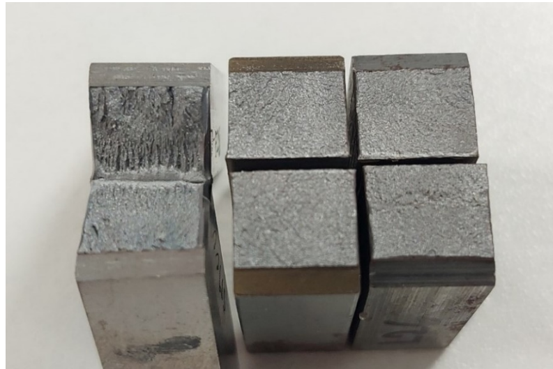
Figure 5.47. Fractured Charpy impact specimens at -60 °C. BM (left), AW (centre) and HT (right).
