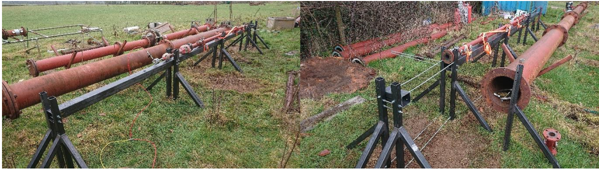
Figure 36: Shock tube mounted at farm test site (smaller tube secured with ratchet straps, larger tube was not part of the experiment). Left image shows the shock tube driver section, whilst right image shows the test section and sample mounting region. The shock tube was designed by Aber Shock and Detonation Research Ltd. who also provided the test site and consumables and operated the equipment. Preparation and transportation of the tube and related equipment for testing was aided by a team of post-graduate students from Swansea University. The mounting system for the tube and sample is a custom integrated design.
