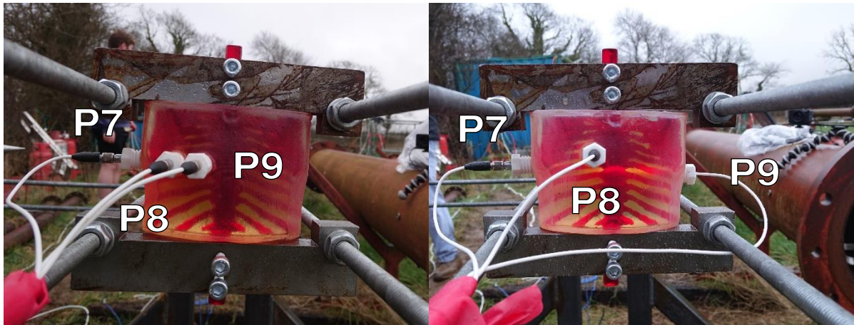
Figure 45: Experimental arrangement of the thorax models in the primary position (rear view). The left model is referred to as the propagation model, the right is referred to as the scatter model. Sensors are indicated on the images with sensor P7 notably being in a consistent position in both samples. In the second thorax model, there is significantly increases embedment depth of sensors P8 and P9, the latter of which can be faintly observed in the image. Wires were secured to the threaded bar to limit motion and collisions with structures which may interfere with the signal received.
