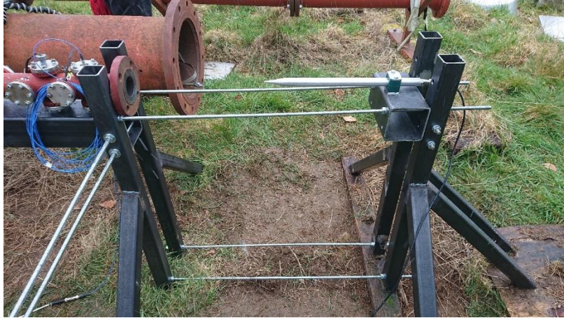
Figure 39: Experimental arrangement of pencil probe in the primary position. Pencil probe is secured with a pipe clamp with grease applied to the sensor to mitigate thermal effects.
