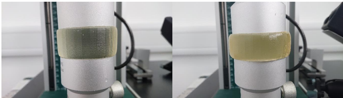
Figure 29: Compression testing of the cylindrical samples of Agilus-30 (left) and Agilus-706B (right). Despite applying lubrication using vegetable oil, significant barrelling can be observed when testing both samples.
