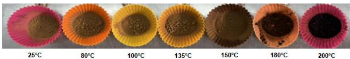
Figure 5: Kraft lignin samples conditioned at different production temperatures.
