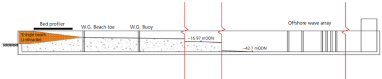
Figure 5.4 Flume set-up (HR Wallingford Modelling Hall)
