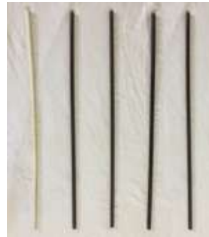
Figure 4. Developed Rods- PLA(a); PLA/BS1(b); PLA/BS2(c); PLA/BS3(d); PLA/BS4(e)
