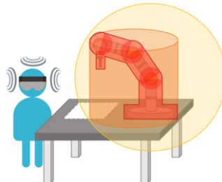
Figure 4: Design for situation awareness and set-up for HRC task.
