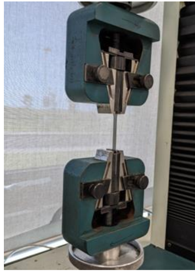
Figure 2.4 Example of a AISI 304 specimen under tensile test.
