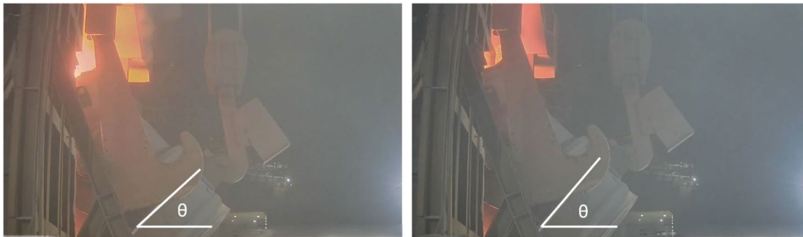
Fig. 13 Example HM charging angle measurement at time t and t+n
