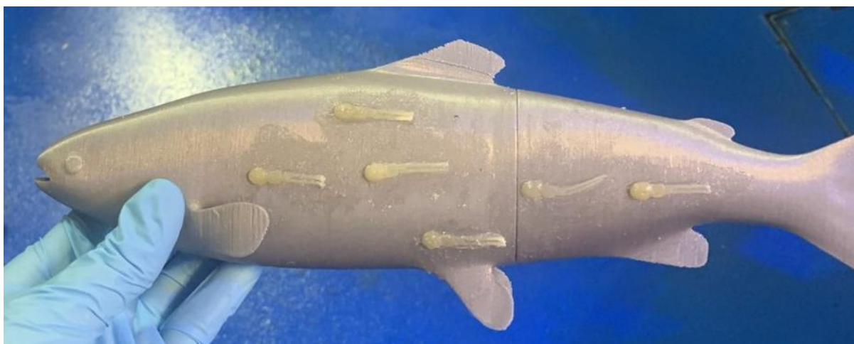
Figure 3.3. 3D-printed salmon model (designed with Atlantic salmon smolt measurements) with latex sea lice attached to side with marine grade silicone.
