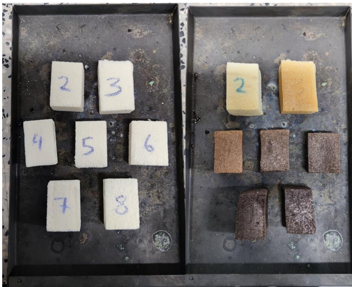
Figure 2.21. Photographs of unheated foam samples (left) and after heating (right). Sample numbers from 2-8 correspond to final heating temperatures of 200 °C, 250 °C, 300 °C, 350 °C, 375 °C, 400 °C, and 425 °C in ascending order.
