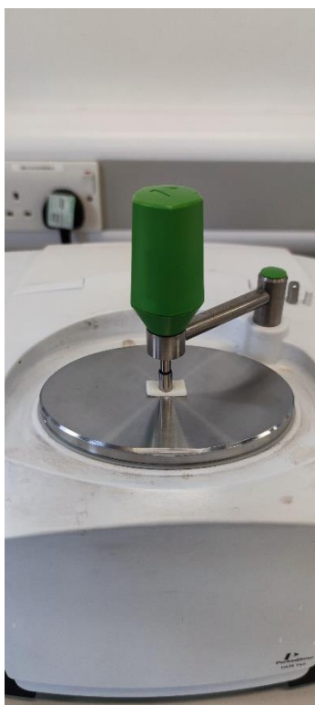
Figure 2.24. Positioning of foam sample in contact with ATR crystal.
