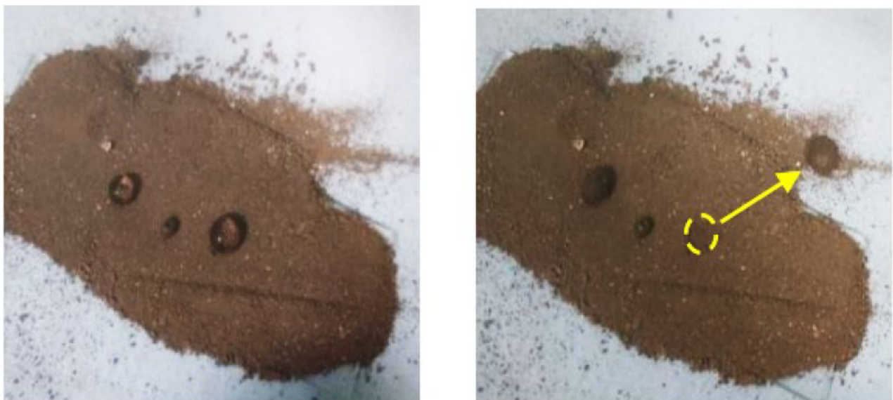
Figure 5.13 Image of liquid marbles being formed on ESP dust.
