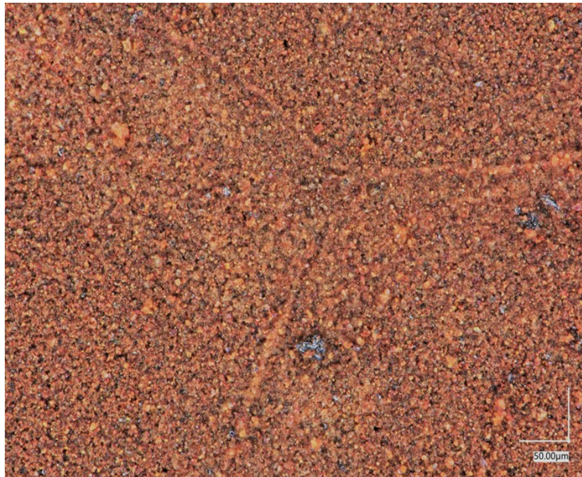
Figure 4.30 Keyence microscope image and 3D map of chicken wire structure on TX-100 light surface. 50 µm scale for image and 14.61 µm scale for 3D map.
