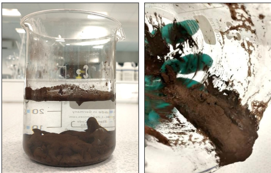
Figure 5.14 Images from ESP dust water washing test. Showing hydrophobic behaviour in water before agitation (left), with post-washing dry ESP dust after washing (right).
