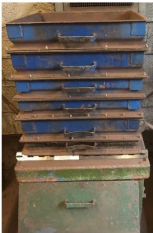
Figure 3.11 Mechanical sieve used for particle size distribution analysis of sinter.
