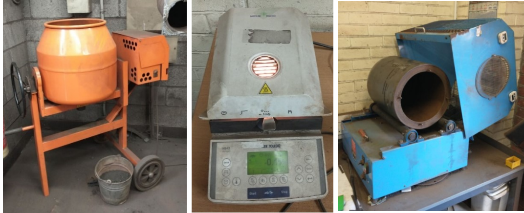
Figure 3.6 Altrad Belle Maxi 140 Cement Mixer (left), Mettler Toledo HB43 Halogen Moisture Analyser & Gladstone Engineering G94 Special Granulator (right).
