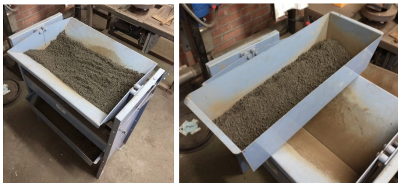
Figure 3.7 Gilson SP-1 Universal Splitter riffle box being used to split granulated samples (left) & one tray after splitting (right).
