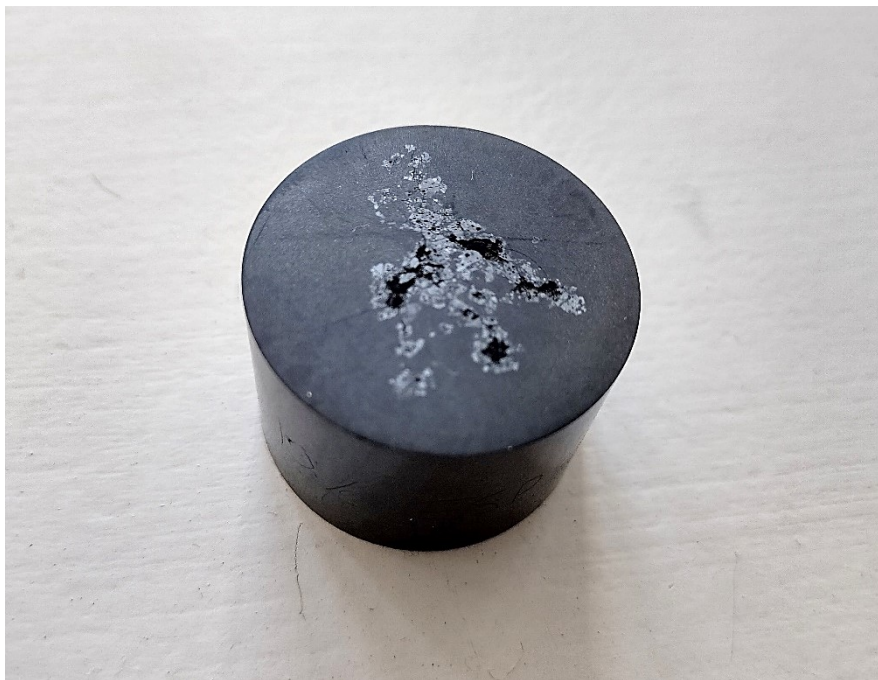
Figure 3.15 Resin mounted sinter sample after polishing process.
