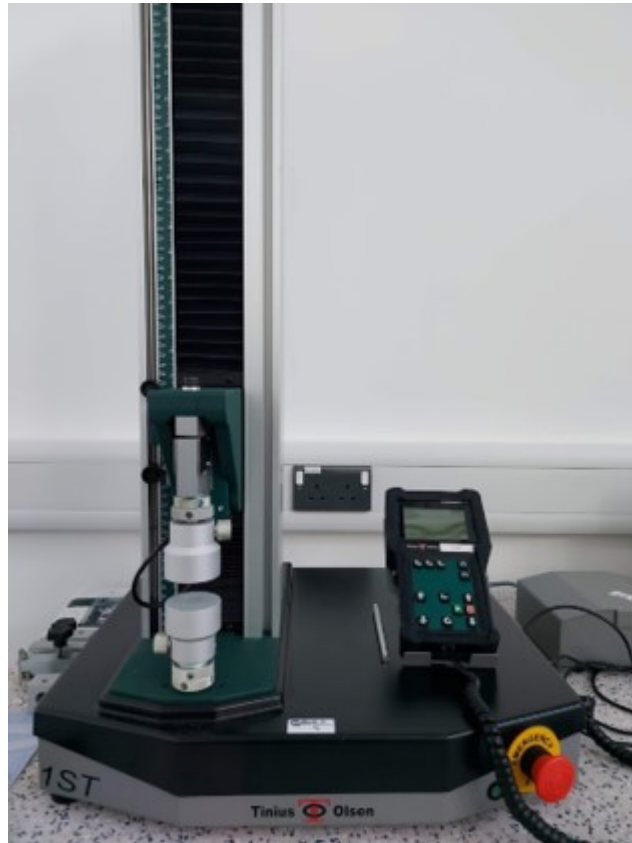
Figure 2.11: Tinus Olsen force testing machine set up for mechanical testing of microneedles
