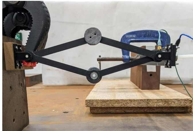
Figure 43: A photograph of the single-stage IA coupled to a cantilever beam, with 12g of proof mass at each specified joint of the mechanism.
