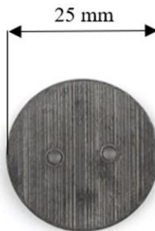
Figure 20: An image of one 12g circular lead disk, with a diameter of 25mm [125]
