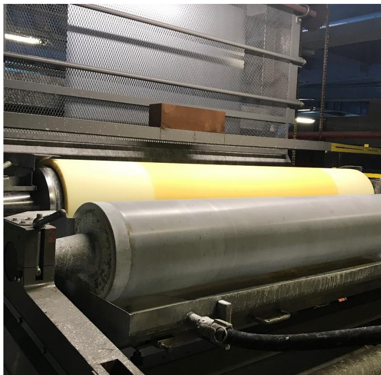
Figure 3. Chemcoater apparatus at ZODIAC galvanising line, Llanwern.
