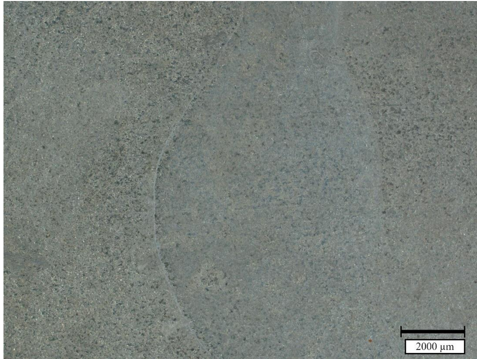
Figure 18. Digital microscopy of PrimeCoat coated HDG surface at \times 20 magnification (2mm scale).
