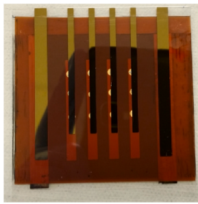
Fig. 7. AlSat-1N TFSC payload 4 cell test structure contact plate (gold on 100 μm thick QST glass).
