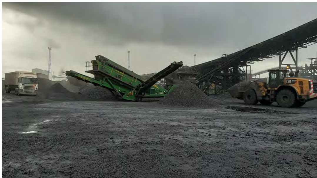
FIGURE 6.2: McCloskey S190 coke screener operating at TATA Steel
