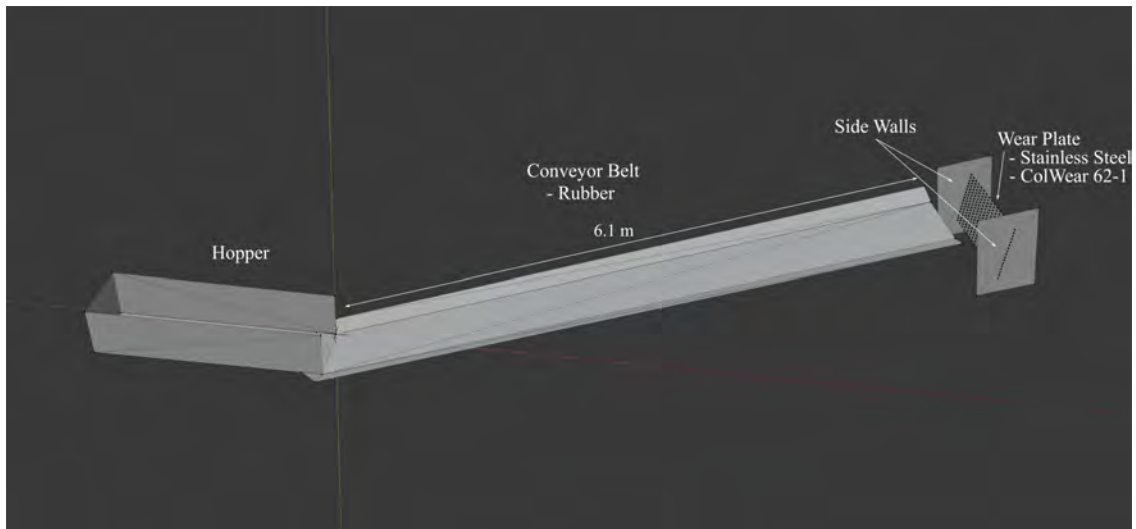
FIGURE 6.3: 3D model created to simulate the coke screener displayed in Blender
