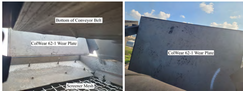
FIGURE 6.7: Coke Screener plate trial week 0
