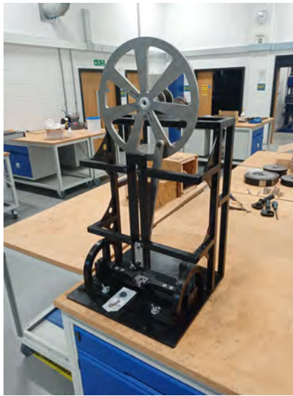
FIGURE B.1: Repetitive Impact Rig build in workshop
