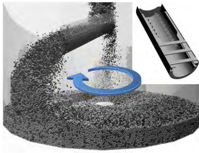
FIGURE 1.2: Blast furnace simulation carried out investigating chute design in Holmes' work [2]
