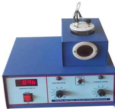
Figure 2.2. Melting point apparatus
