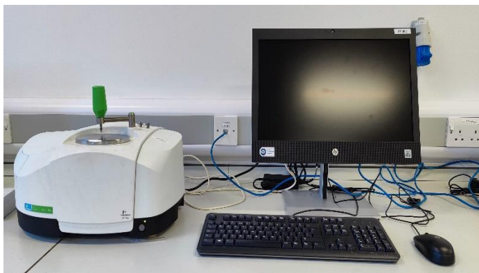
Figure 2.1. PerkinElmer UATR Two was used for the analysis of Intermediate #1, Intermediate #2 and the Ligands
