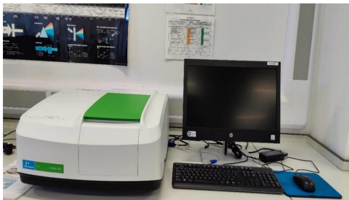
Figure 2.6. Perkin-Elmer 25 UV-Vis spectrophotometer was used for the analysis of the colloidal gold nanoparticles
