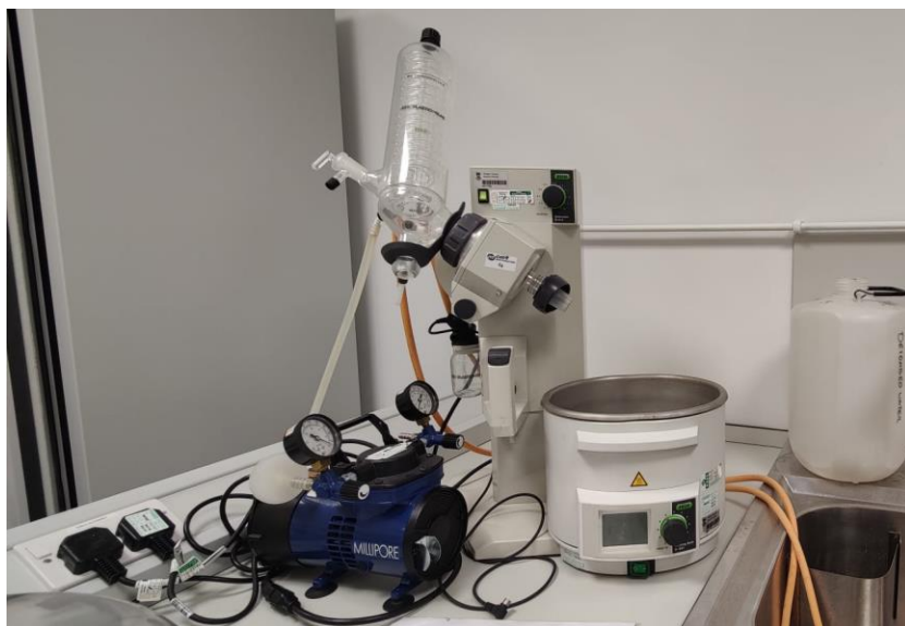
Figure 2.3. Instrumentation of the rotary evaporator
