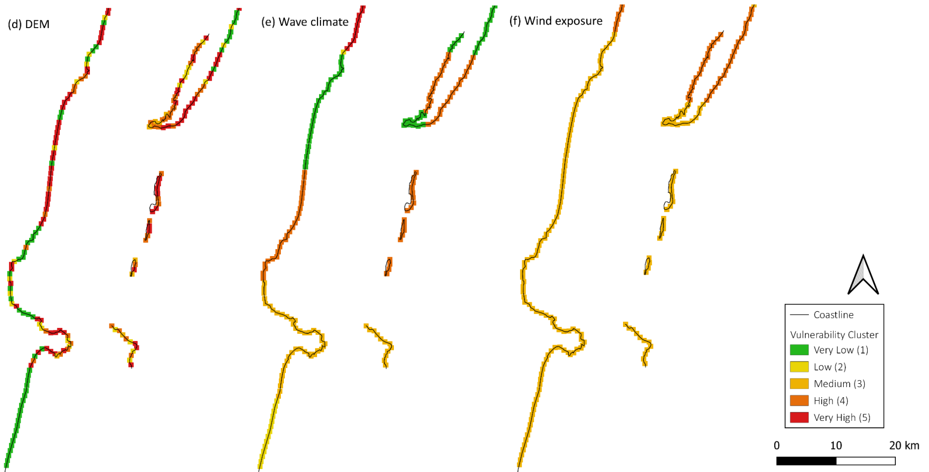
Figure 52: Relative vulnerability ranking of coastal segments for each parameter based on KMeans clustering.
