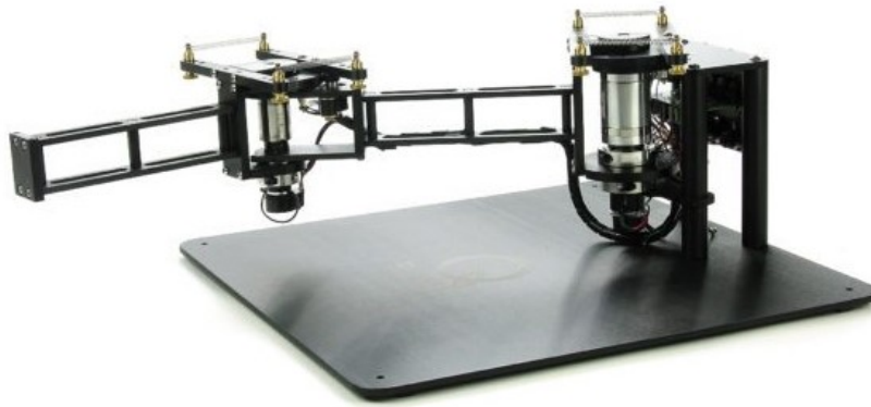
Figure 1: Quanser Robot with two Degrees of Freedom (DoF)
