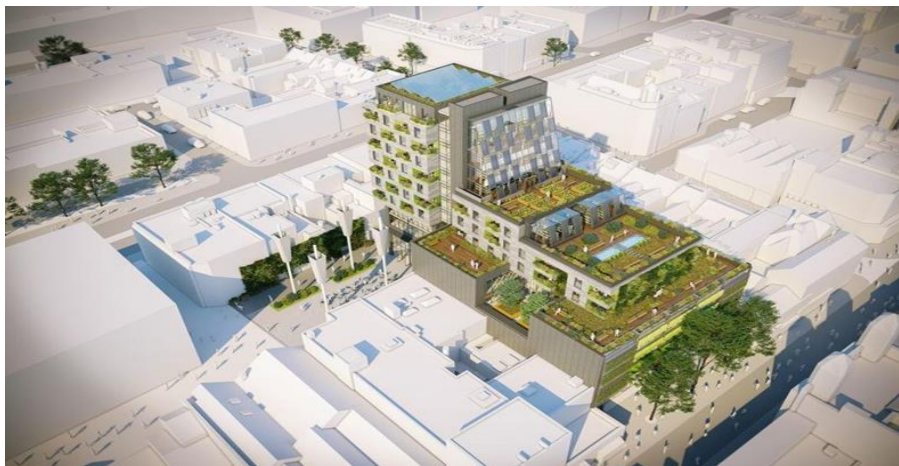
Figure i.ii Conceptual building design in Swansea, displaying the key biophilic aspects of living walls and the greenhouse systems. ( https://www.biophilicliving.co.uk/about/ )
