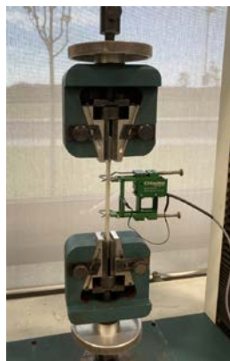
Figure 32. Tensile test set up with extensometer
