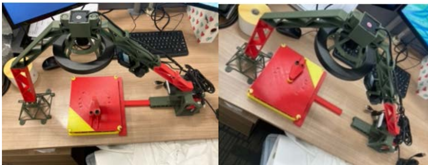
Figure 81. Inspection system. Product central to camera (left). Base fixture fixed in place (right).
