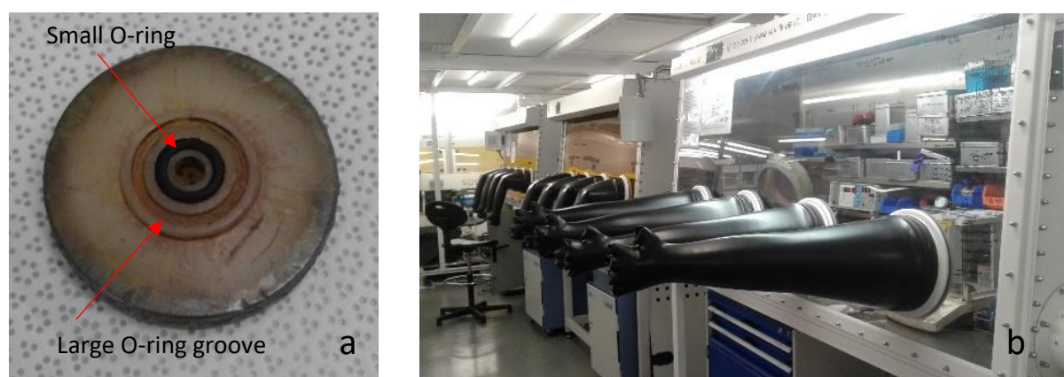
Figure 21 - a Spin-coater chuck with detail on O-ring size. b Nitrogen atmosphere glove box used for spin-coating.
