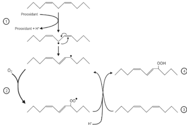
Figure 5. The mechanism of lipid peroxidation, showing (1) initiation, (2,3) propagation and (4) termination. During initiation, the radical is stabilised by forming a conjugate diene due to rearrangement. This means when the peroxy radical is formed during propagation, the peroxy group attaches to C_4 .
