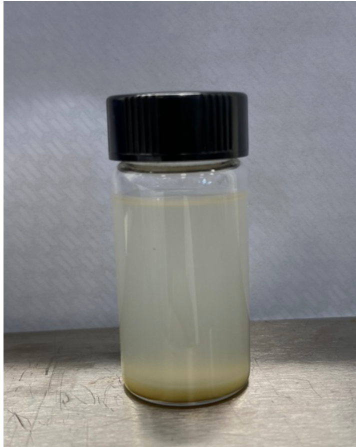
Figure 29: Image of functionalized Al 2 O 3 (5 nm) nanoparticle after being dispersed in 2-propanol ready to be sprayed onto substrates. Source: Author's picture based on the experimental setup
