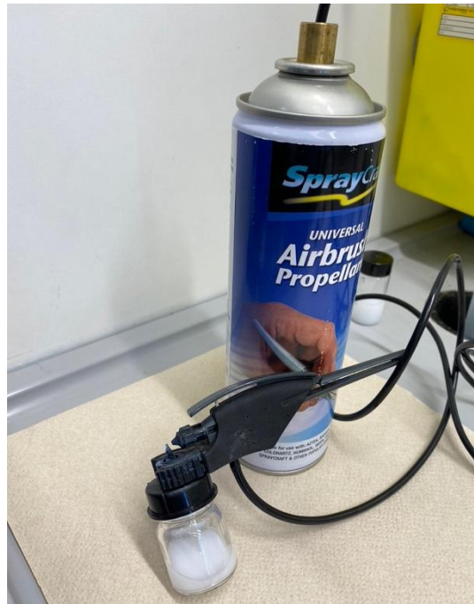
Figure 27: Image of functionalised Al_2O_3 (13nm) nanoparticles dispersed on 2-propanol, ready to be spray coated onto substrates. Source: Author's picture based on the experimental setup
